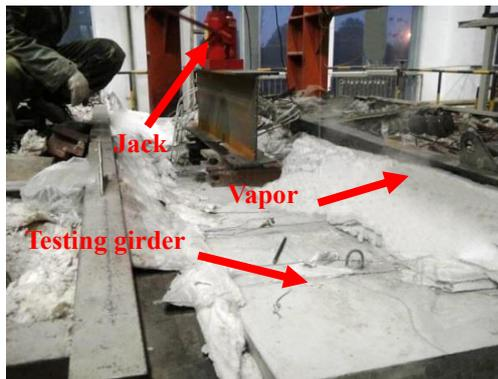
Fig. 5 Picture showing of the testing girder
