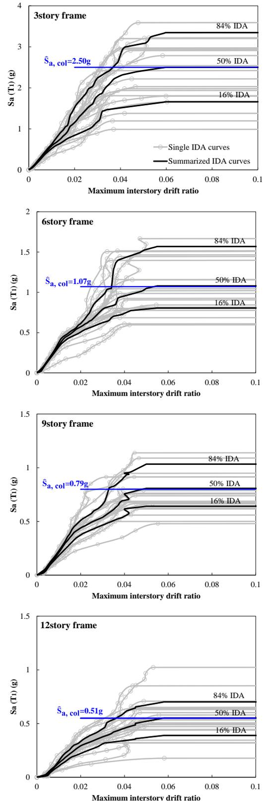
Fig. 5 IDA results for the example structures subjected to the set of twenty ground motion records when the maximum interstory drift ratio is considered as the EDP
