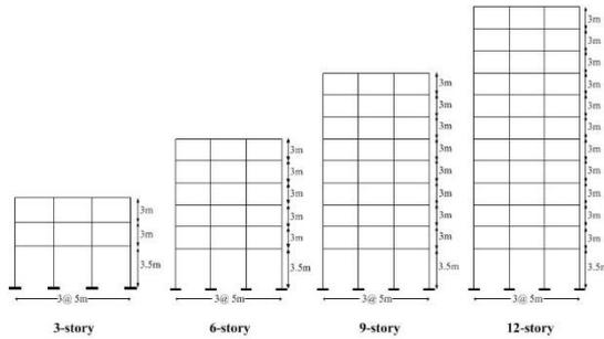
Fig. 3 Elevation view of the structural models considered for this study
