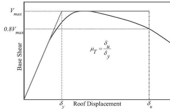
Fig. 2 Definition of parameters required from bilinear idealized pushover curve in the method proposed by Hamidia *et al.* (2013)
