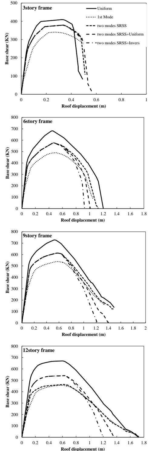
Fig. 7 Pushover curves for the studied RC frames produced by four different lateral load patterns
