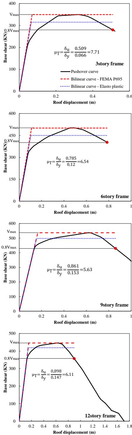
Fig. 10 Bilinear representation of pushover curves based on EPP and FEMA-P695. Target ductility demands required by the Hamidia *et al.* method are also shown in the plots
