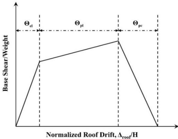
Fig. 1 Definition of parameters required from idealized pushover curve for generic structural models in the method proposed by Shafei *et al.* (2011)
