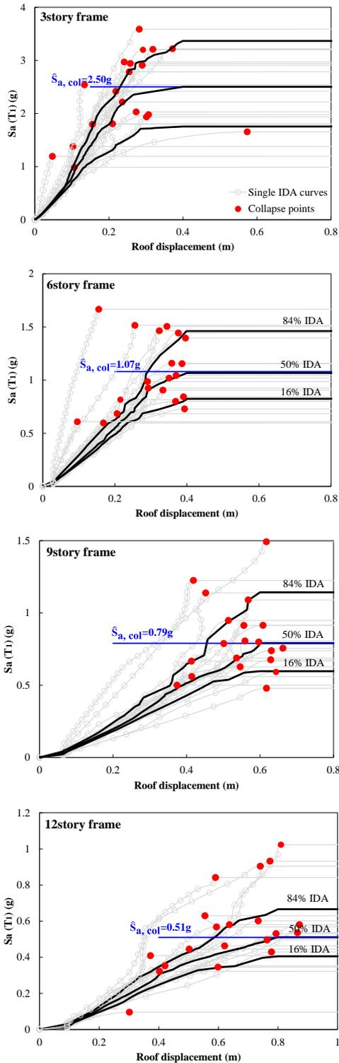
Fig. 6 IDA results for the example structures subjected to the set of twenty ground motion records when the roof displacement is considered as the EDP. The collapse points are shown by filled circles
