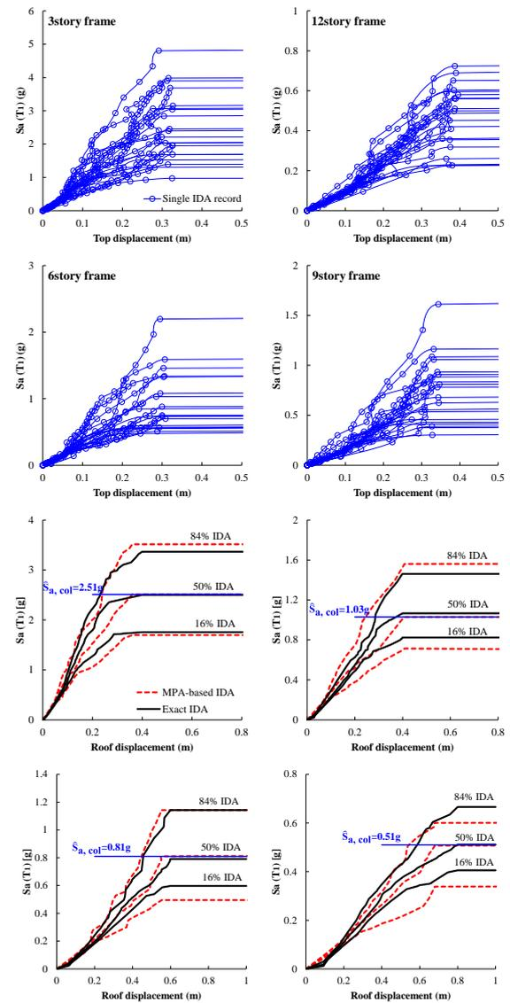
Fig. 9 IDA curves for the first-mode SDOF systems and the corresponding MPA-based IDA results for the example buildings
