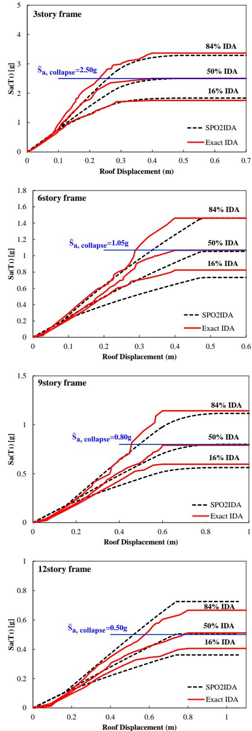
Fig. 8 Sixteen, 50 and 84% fractile IDA curves for the 3-, 6-, 9- and 12-story example structures from nonlinear RHA (exact) versus SPO2IDA approximate procedure
