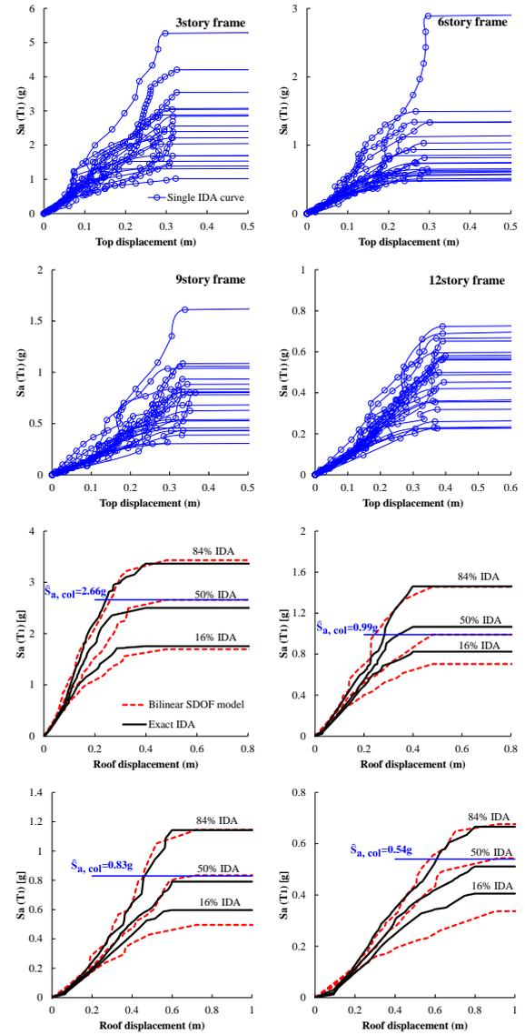
Fig. 11 IDA curves for the equivalent SDOF systems with backbone curves displayed in Fig. 10 (dotted curves), and the corresponding IDA results for the example buildings. The median collapse capacities are also shown in the plots
