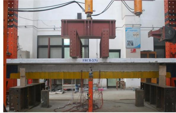
Fig. 4 Test device
