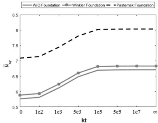
Fig. 11 Effect of translational restraint stiffnesses on the nondimensional shear buckling load ( $k_r = 0$ )
