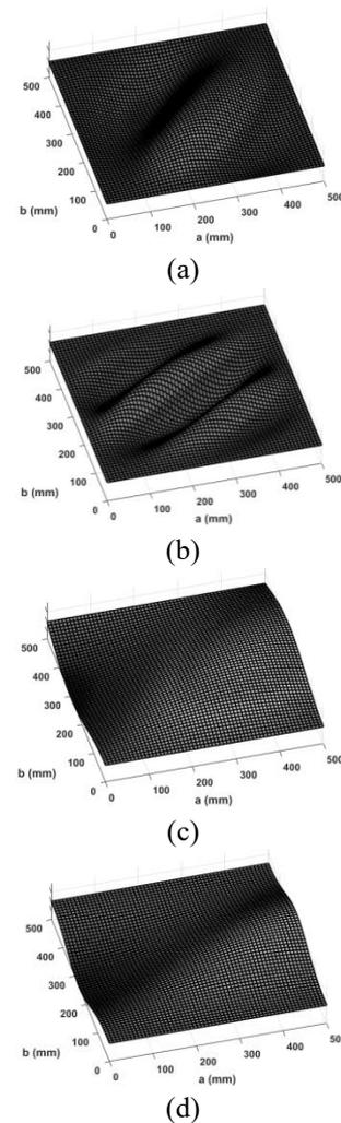
Fig. 3 The buckled shapes of the laminated square plates for MATLAB programming: (a) 4S, (b) 4C, (c) 2F2S, (d) 2F2C
