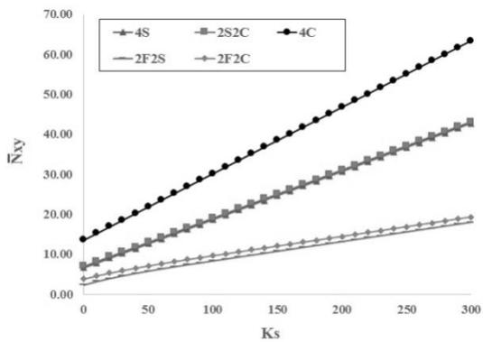
Fig. 8 Effect of the foundation parameter ( $K_s$ ) on the nondimensional shear buckling load
