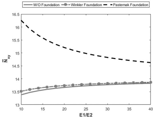
Fig. 7 Effect of the modulus ratio ( $E_1/E_2$ ) on the nondimensional shear buckling load
