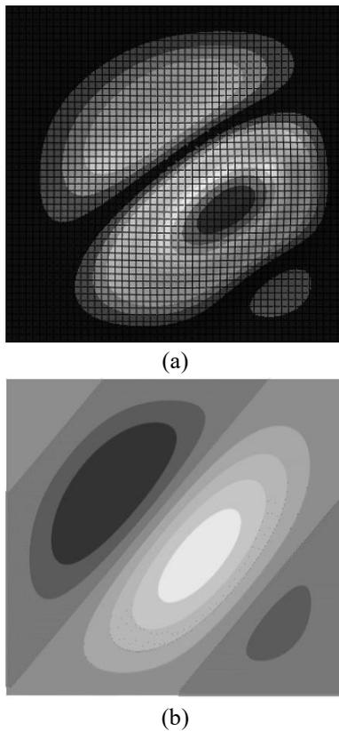
Fig. 2 Comparisons of the buckled shapes for simply supported laminated square plate for MATLAB programming (a) and finite element solution (b)
