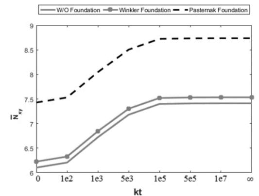
Fig. 12 Effect of translational restraint stiffnesses on the nondimensional shear buckling load ( $k_r = \infty$ )
