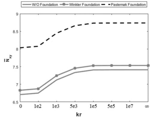
Fig. 10 Effect of rotational restraint stiffnesses on the nondimensional shear buckling load ( $k_t = \infty$ )
