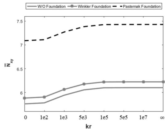
Fig. 9 Effect of rotational restraint stiffnesses on the nondimensional shear buckling load ( $k_t = 0$ )
