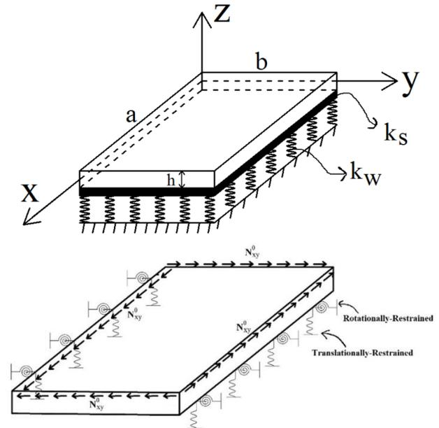
Fig. 1 A laminated composite plate resting on Pasternak foundation
