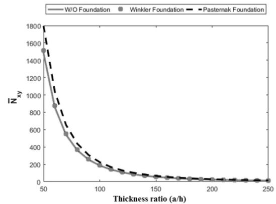
Fig. 6 Effect of thickness ratio (a/h) on the nondimensional shear buckling load for simply supported boundary condition
