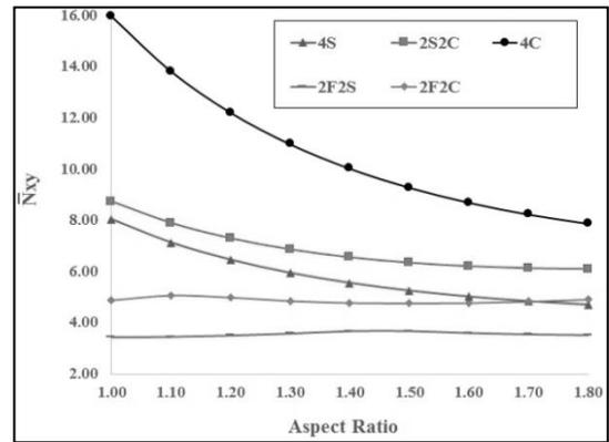
Fig. 5 Effect of plate aspect ratio and boundary conditions on the nondimensional shear buckling load with Pasternak foundation
