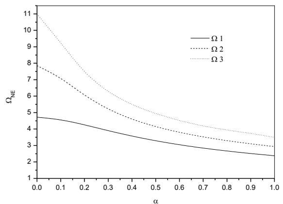
Fig. 3 small scale effect on different frequency modes for Clamped beam and ( $k_{win}=0.1, L/d=10$ )
