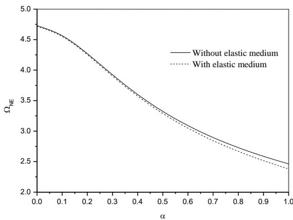
Fig. 5 The effect of elastic medium on first non-dimensional frequency of a short-SWCNT for clamped ends with different parameter  $\alpha$  and  $L/d=10$
