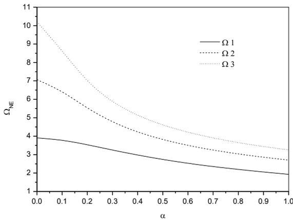
Fig. 4 small scale effect on different frequency modes for Clamped simply supported beam and ( $k_{win}=0.1$ ,  $L/d=10$ )
