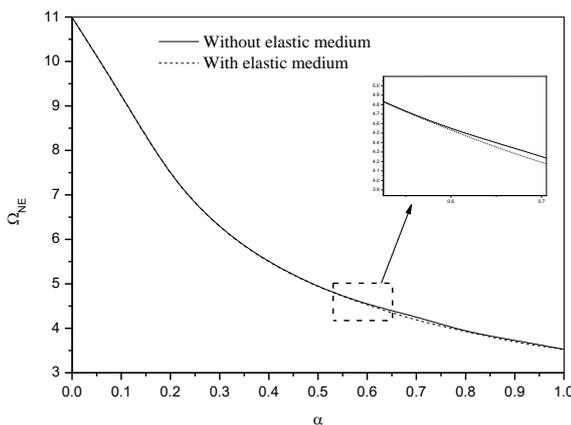
Fig. 6 The effect of elastic medium on third non-dimensional frequency of a short-SWCNT for clamped ends with different parameter  $\alpha$  and  $L/d=10$
