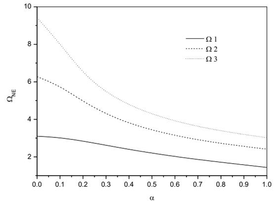
Fig. 2 small scale effect on different frequency modes for simply supported beam and ( $k_{win}=0.1, L/d=10$ )
