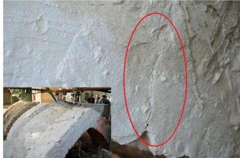
(b) Cracks in the vault under the load of 171 kN
