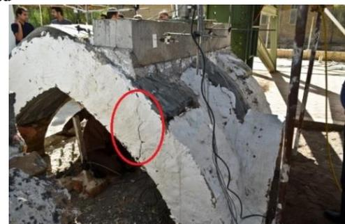
(b) Cracks in the vault under the load of 245 kN
