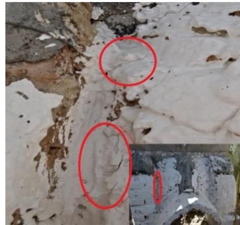
(b) Cracks at the junction of rib cover to the vault under the load of 235 kN
