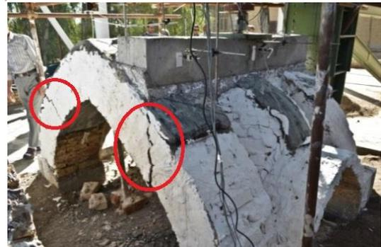
(b) Place of cracks in the vault, reinforced structure
