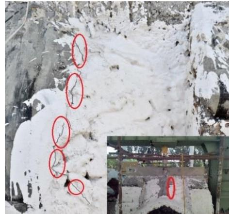
(a) Crack around the reinforced area with FRP under the load of 215 kN
