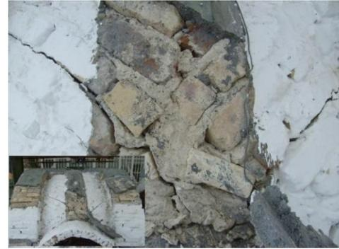
Fig. 18 Crack in the rib cover of reinforced structure after loading
