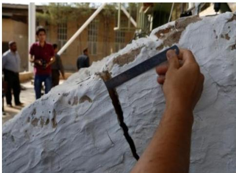
(d) Increase the width of the cracks in the left vault to 2 cm
