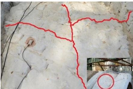
(a) Cracks with a cross shape in the rib cover under a load of 137 kN
