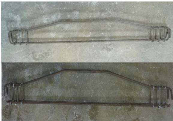
Fig. 5(a) Reinforcement details
