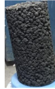
Fig. 2 Photo of cylindrical pervious concrete specimen using RAP
