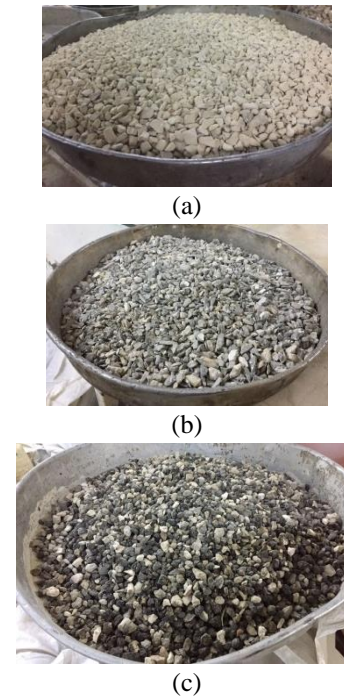
Fig. 1 Photo of coarse aggregate used: (a) NA; (b) RCA; (c) RAP
