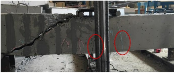
Fig. 13 Flexural cracking of specimens B120-12-90-M
