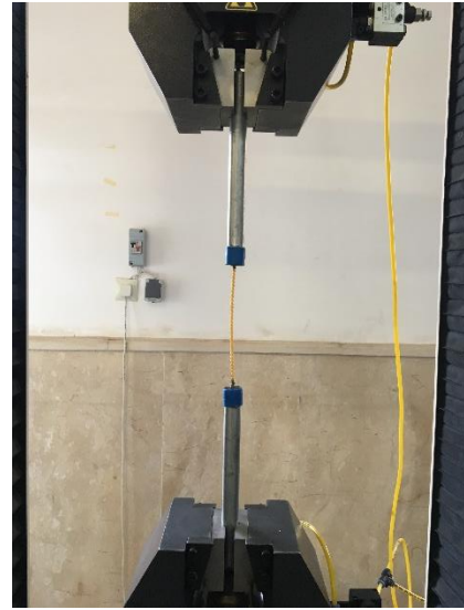
Fig. 7 Tensile testing of a GFRP bar
