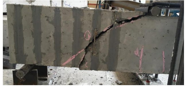
Fig. 10 Cracking pattern and failure mode of specimen B100-15-90
