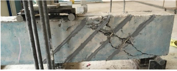
Fig. 11 Cracking pattern and failure mode of specimen B150-15-45
