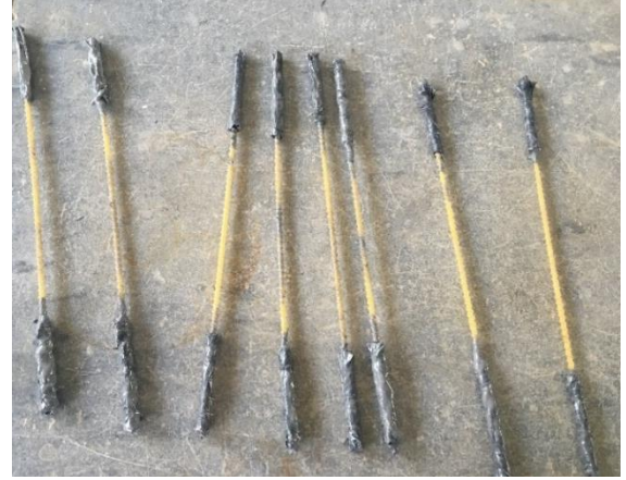
Fig. 3 Illustration of the manually strengthened GFRP bars
