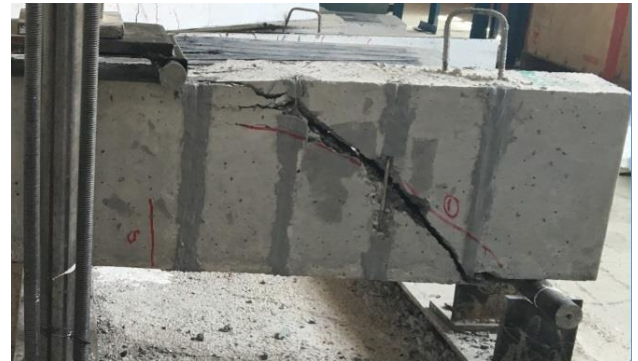
Fig. 11 Cracking pattern and failure mode of specimen B150-15-90
