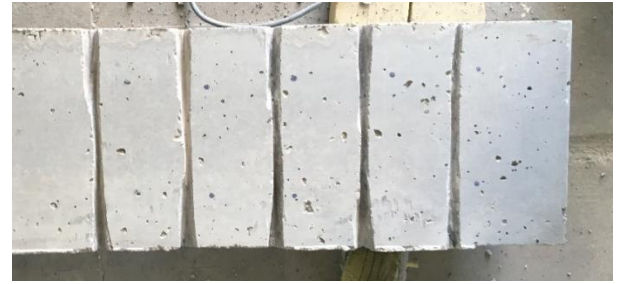
Fig. 4 Grooves carved for MNSM strengthening method
