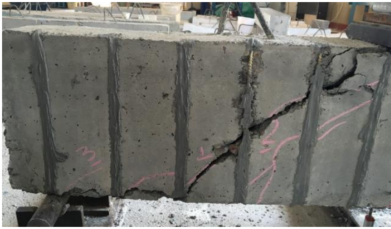
Fig. 9 Cracking pattern and failure mode of specimen B120-12-90
