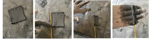
Fig. 2 Manufacturing process of the manually strengthened GFRP bars
