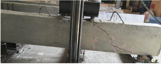
Fig. 8 Cracking pattern and failure mode of the control specimen, BC
