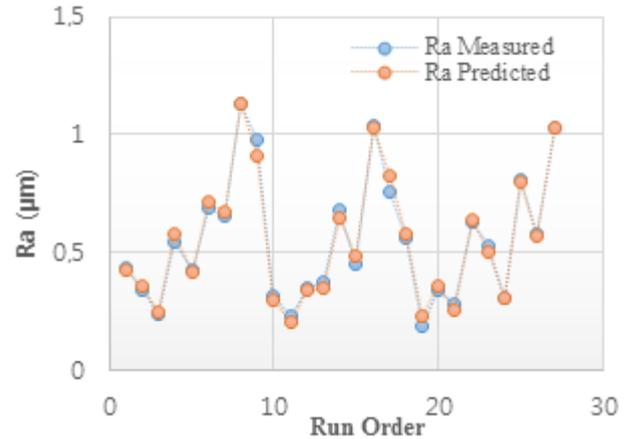
Fig. 5 Comparison of the measured and estimated surface roughness (Ra)
