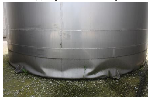
(b) diamond shape buckling
