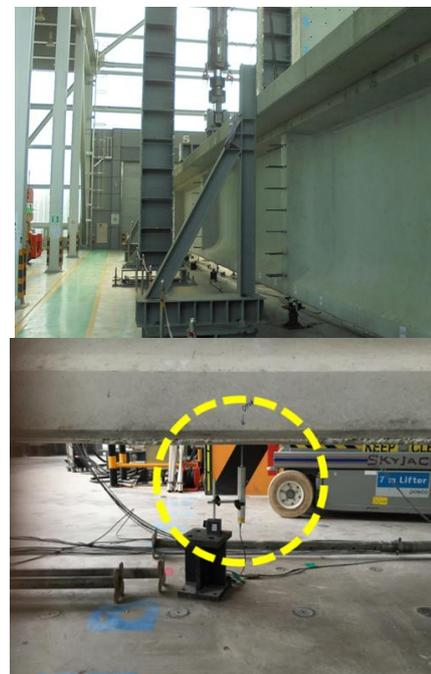
Fig. 6 Experimental loading test and measurement of displacement at the center of girder
