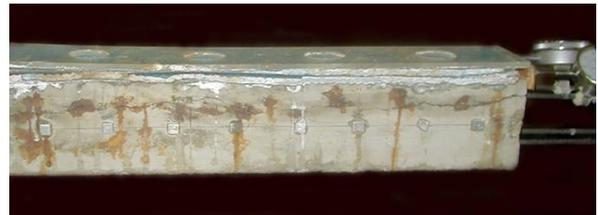
Fig. 2 Beam IV during the accelerated corrosion process
