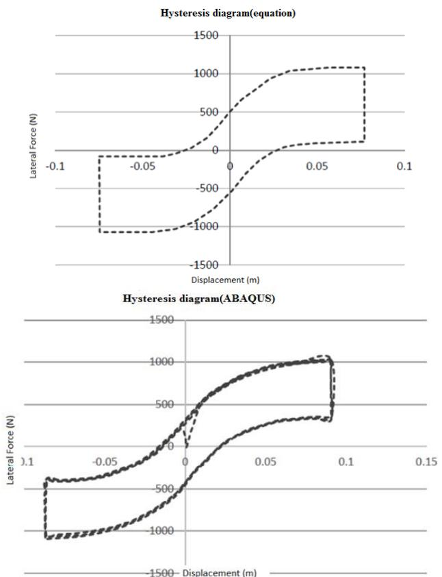
Fig. 6 Hysteresis diagram of DVFPI isolator, unequal geometry and equal friction
