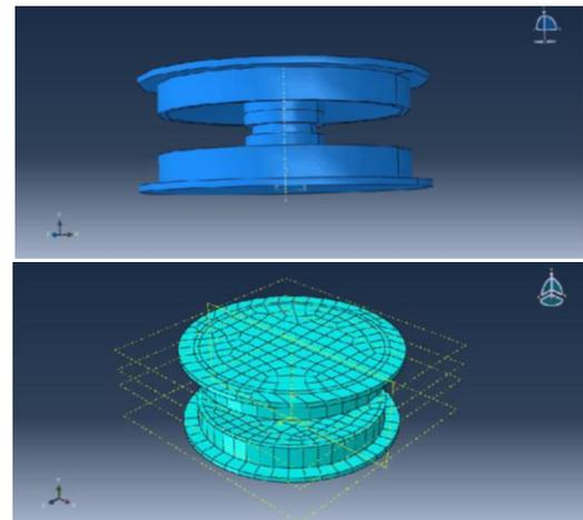
Fig. 3 The modeled isolator in ABAQUS software
