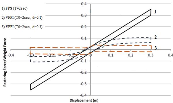
Fig. 10 The effect of parameter  $d$  on the restoring force relative to displacement, compared with DCFP isolator
