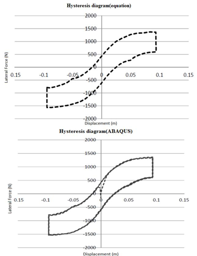
Fig. 5 Hysteresis diagram of DVFPI isolator, unequal geometry and friction
