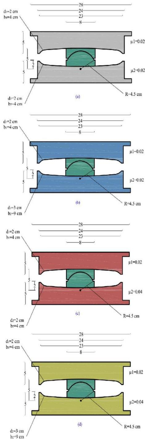
Fig. 2 Sample DVFPI isolators modeled, (a) with equal friction and geometry, (b) with equal friction and unequal geometry, (c) with unequal friction and equal geometry and (d) with unequal friction and geometry
