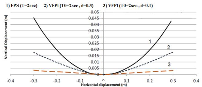
Fig. 9 Effect of parameter  $d$  on vertical displacement, compared to DCFP isolator
