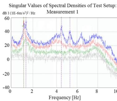
(a) Singular values of spectral densities matrices obtained from EFDD method
