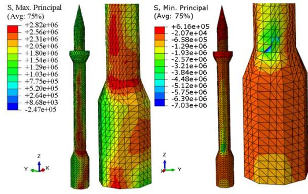
Fig. 17 Maximum and minimum principal stresses in minaret (Pa)
