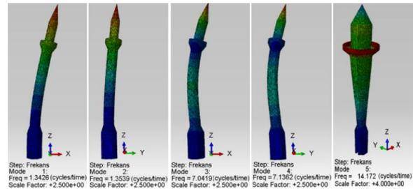
Fig. 6 Mode shapes and frequency values obtained from the initial FE model
