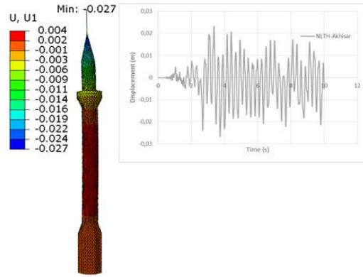
Fig. 14 Displacements of the minaret subjected to Akhisar earthquake (m)
