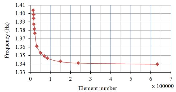
Fig. 5 Frequency and mesh size convergence graphic
