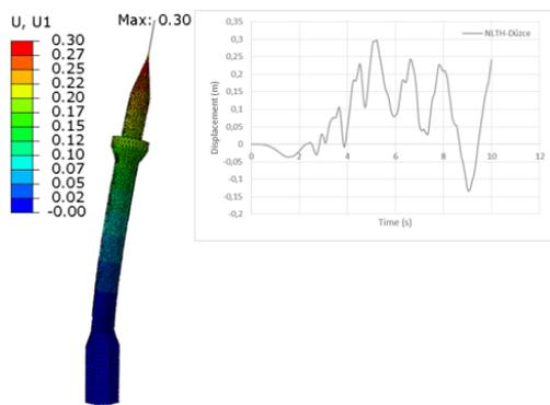
Fig. 16 Displacements of the minaret subjected to Düzce earthquake (m)
