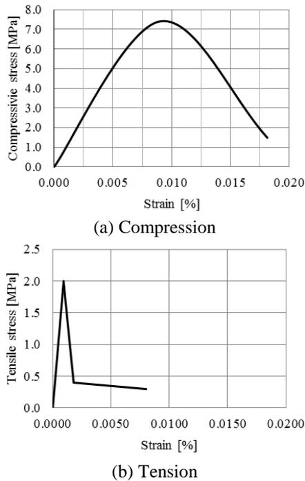
Fig. 9 The material models used for masonry
