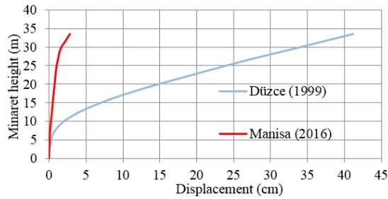
Fig. 12 Lateral displacements throughout the height for LTH analyses
