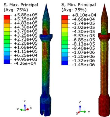
Fig. 15 Maximum and minimum principal stresses of minaret (Pa)
