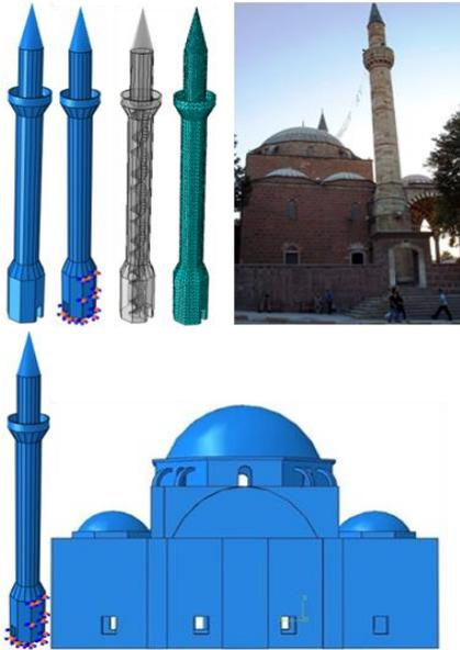
Fig. 4 Three-dimensional solid model and FE model of minaret
