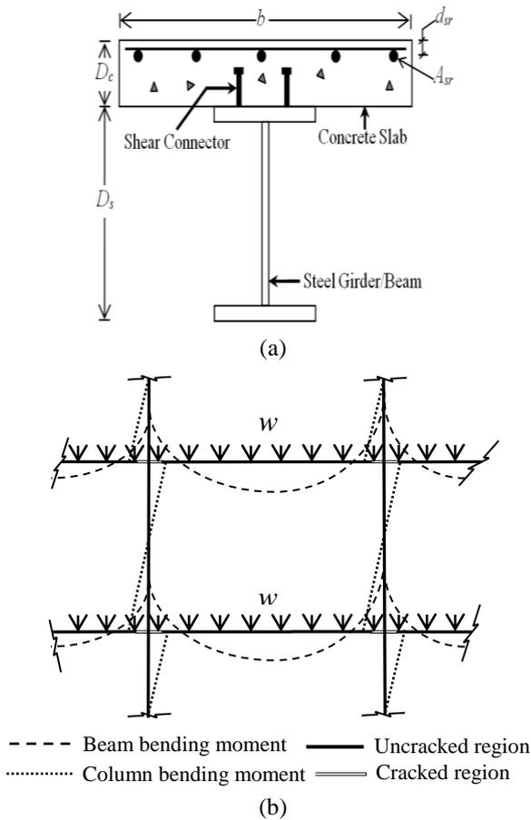
Fig. 1 (a) A Typical cross-section of a composite beam and (b) a typical segment of a composite frame with loads, bending moments, and possible cracked and uncracked regions
