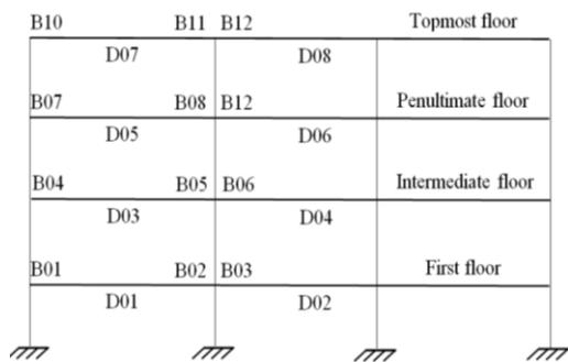
Fig. 5 Representative three bay four storey frame for data generation showing the designations of neural networks (only significant characters in the designations of neural networks are shown e.g. B01 for NetB01 and D01 for NetD01)
