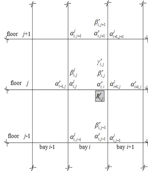
Fig. 3 Input parameters and their positions in a typical floor and bay of a frame for the output parameter  $R_{i,j}^r$
