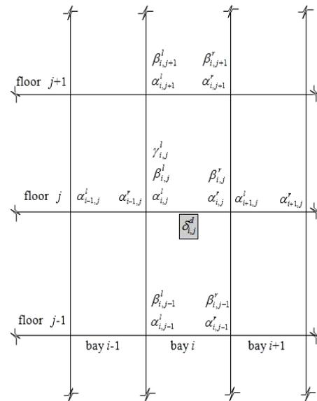
Fig. 4 Input parameters and their positions in a typical floor and bay of a frame for the output parameter  $\delta_{i,j}^d$
