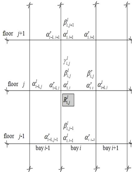
Fig. 2 Input parameters and their positions in a typical floor and bay of a frame for the output parameter  $R_{i,j}^l$
