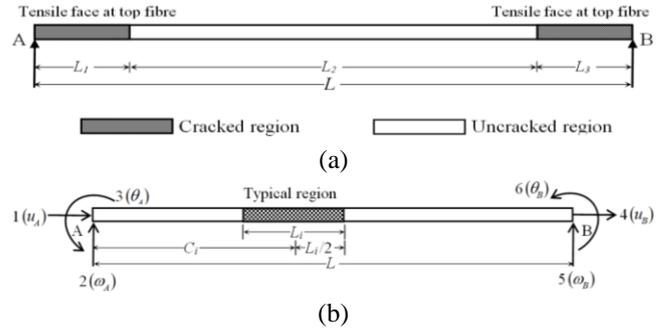
Fig. 6 A cracked span length beam element with (a) cracked and uncracked regions; and (b) degrees of freedom
