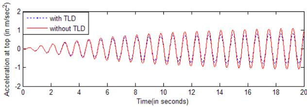
Fig. 11 Structural response history of peak acceleration with and without flat bottom TLD subjected to harmonic base excitation (Structure type Case 3,  $T_s=0.854s$ ,  $\Delta=0.077$ ,  $A_o=0.039\text{ m/s}^2$  and  $\mu=1\%$ )
