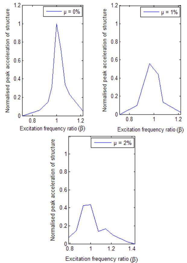
Fig. 16 Normalized peak acceleration for different mass ratio and varied  $\beta$  ratio, for sloped bottom TLD, at beach slope  $30^\circ$  (Structure type Case 3,  $T_s=0.854$ ,  $\Delta=0.077$ ,  $A_o=0.039$  m/s<sup>2</sup>)
