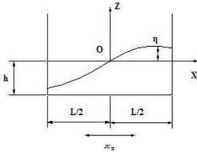
Fig. 6 Dimensions of the rectangular tuned liquid damper
