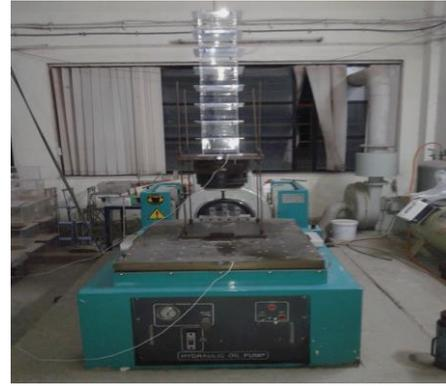
Fig. 8 Test setup, specimen and shaking Table
