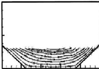
Fig. 2 Streamlines inside a sloped bottom TLD showing no recirculation zone (Morsy 2010)
