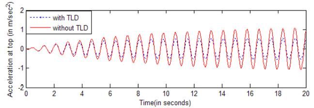
Fig. 14 Structural response history of peak acceleration with and without sloped bottom TLD at beach slope  $30^\circ$ , subjected to harmonic base excitation (Structure type Case 3,  $T_s=0.854s$ ,  $\Delta=0.077$ ,  $A_o=0.039\text{ m/s}^2$  and  $\mu=2\%$ )
