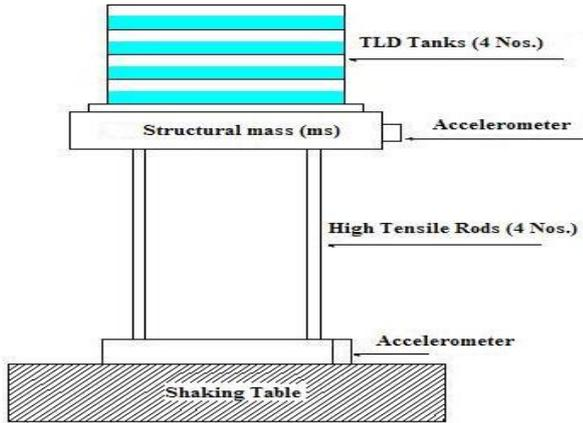
Fig. 7 Schematic diagram of TLD structure model
