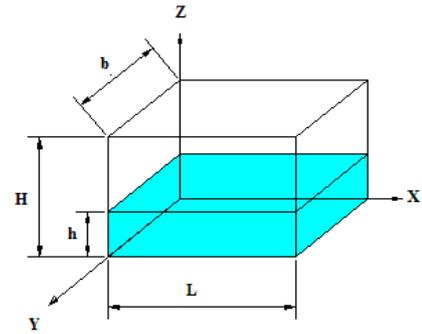
Fig. 3 Schematic of flat bottom TLD
