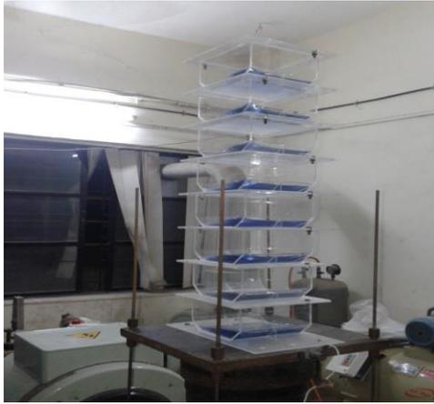
Fig. 10 Eight TLD tanks stacked one over the other (case 3 at beach slope 20°) showing behavior of liquid inside TLD during the test
