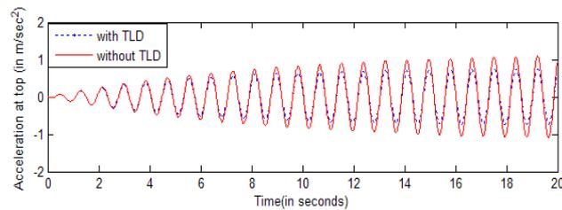
Fig. 13 Structural response history of peak acceleration with and without sloped bottom TLD at beach slope  $30^\circ$ , subjected to harmonic base excitation (Structure type Case 3,  $T_s=0.854s$ ,  $\Delta=0.077$ ,  $A_o=0.039\text{ m/s}^2$  and  $\mu=1\%$ )
