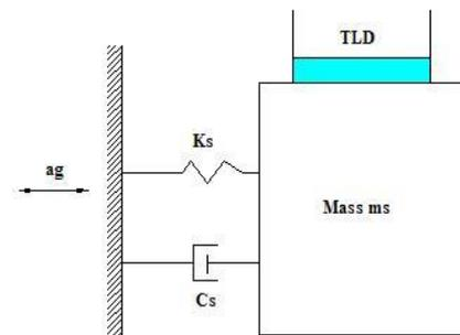
Fig. 5 Schematic of a single-degree-of-freedom structure with a rectangular tuned liquid damper
