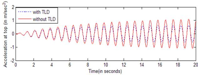
Fig. 12 Structural response history of peak acceleration with and without flat bottom TLD subjected to harmonic base excitation (Structure type Case 3,  $T_s=0.854s$ ,  $\Delta=0.077$ ,  $A_o=0.039\text{ m/s}^2$  and  $\mu=2\%$ )
