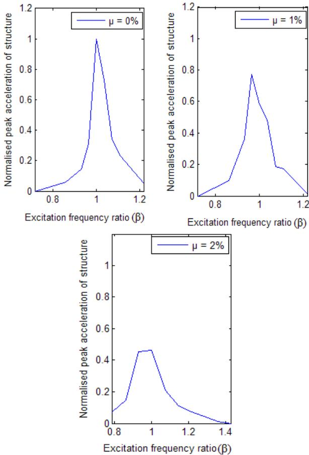
Fig. 15 Normalized peak acceleration for different mass ratio and varied  $\beta$  ratio, for flat bottom TLD, (Structure type Case 3,  $T_s=0.854$  sec.,  $\Delta=0.077$ ,  $A_o=0.039$  m/s<sup>2</sup>)
