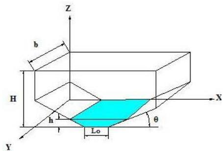
Fig. 4 Schematic of sloped bottom TLD
