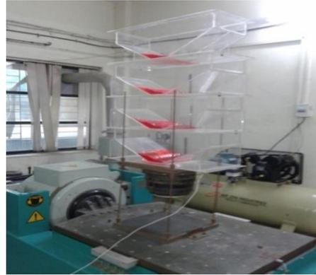
Fig. 9 Behavior of liquid inside TLD during the test
