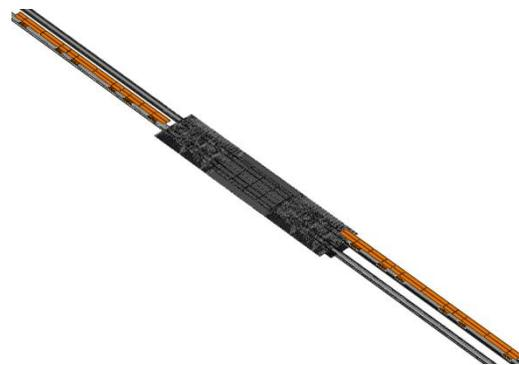
Fig. 17 The 3D FE model of two-way train passing mode
