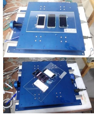
Fig. 4 Smartphones fixed on the shaking table (horizontal (above) and 45 degree (below))
