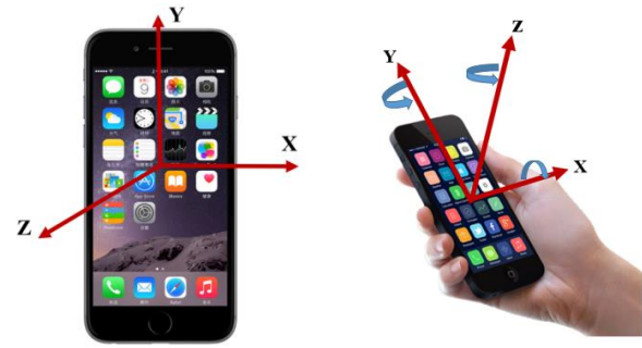
Fig. 2 The coordinate axis of the iPhone and the positive direction of the acceleration sensor
