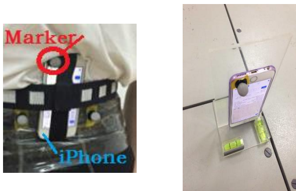
(a) Smartphone on the waist (b) Orientation device Fig. 6 The fixed method
