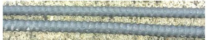
Fig. 2 GFRP bars (9.5 and 11.5 mm in diameter)
