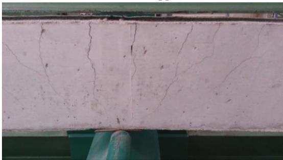
(c) Failure zone at mid-support
