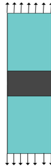
Fig. 4 Applied boundary conditions simulating uniaxial tension
