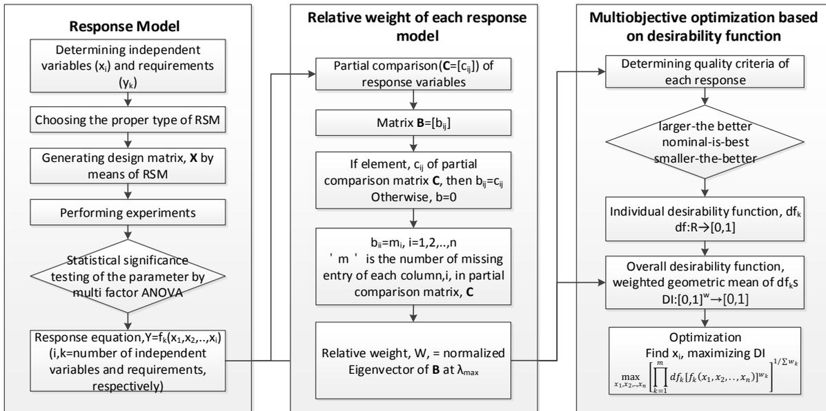
Fig. 1 Proposed RSM based weighted multi-objective optimization procedure
