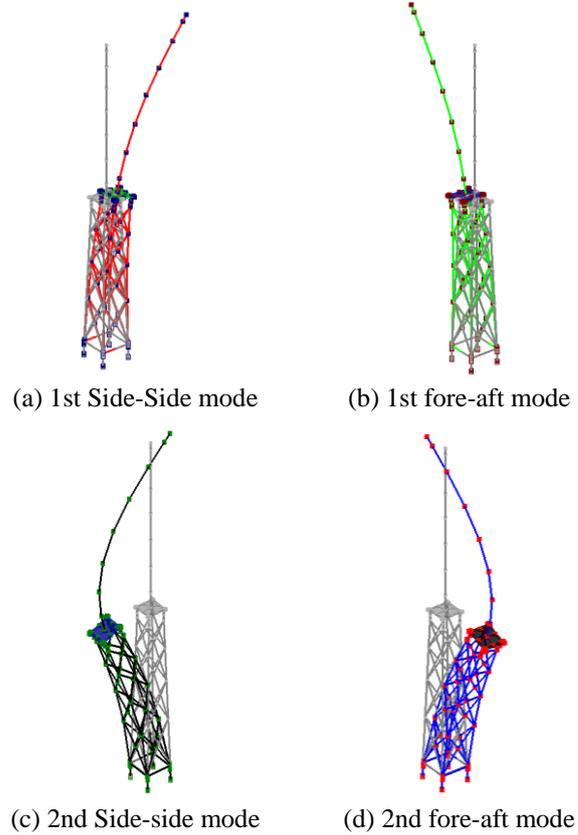
Fig. 4 Mode shape of uncontrolled jacket supported an offshore wind turbine
