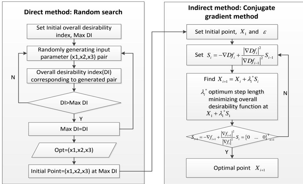
Fig. 2 Composite desirability function for multi-objective optimization
