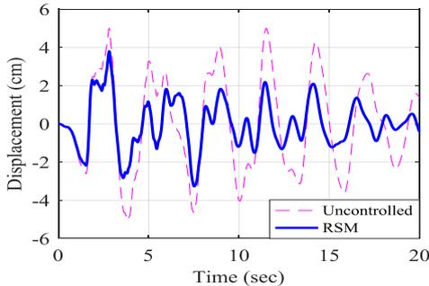
(e) Displacement with/without optimal TMD under Northridge earthquake
