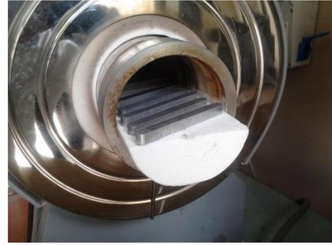
Fig. 4 Beam specimens sintered in the tube oven
