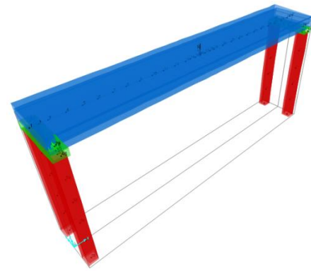
Fig. 11 The 3D finite element model of 40m-span simply supported concrete T-bridge (SAP 2000)
