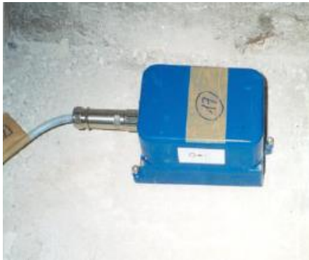
Fig. 6 (a) Ambient vibrations recorded by the accelerometer
