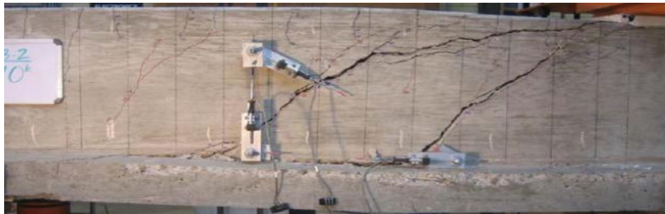
Fig. 9 Beam (24-3-2) at failure load
