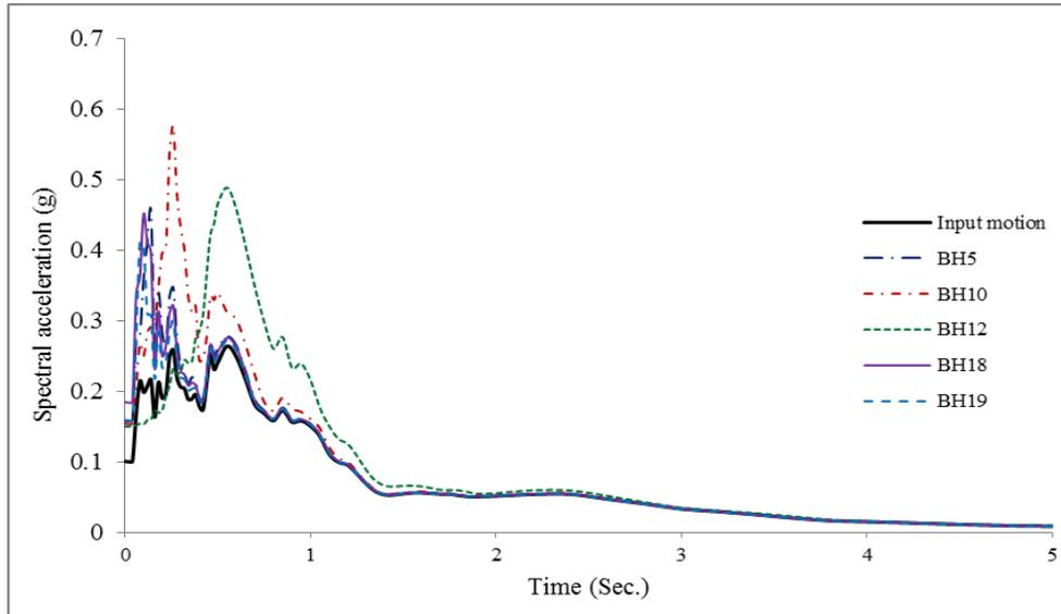
Fig. 6 Response spectra of the surface motion at various bore hole locations
