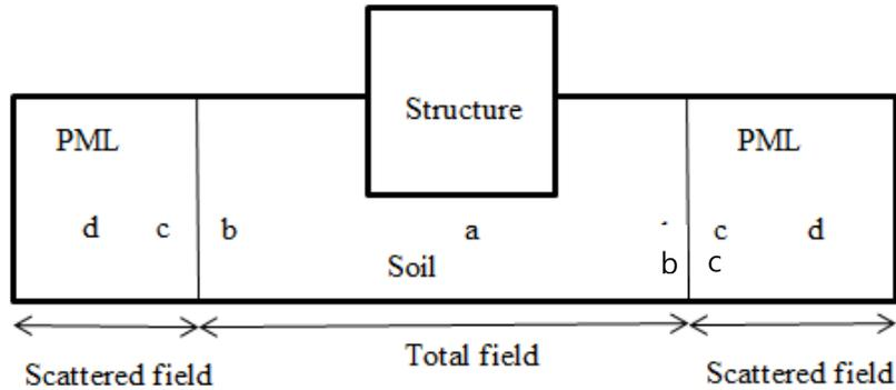
Fig. 1 Partition of DOF's of SSI system (Lee 2006)
