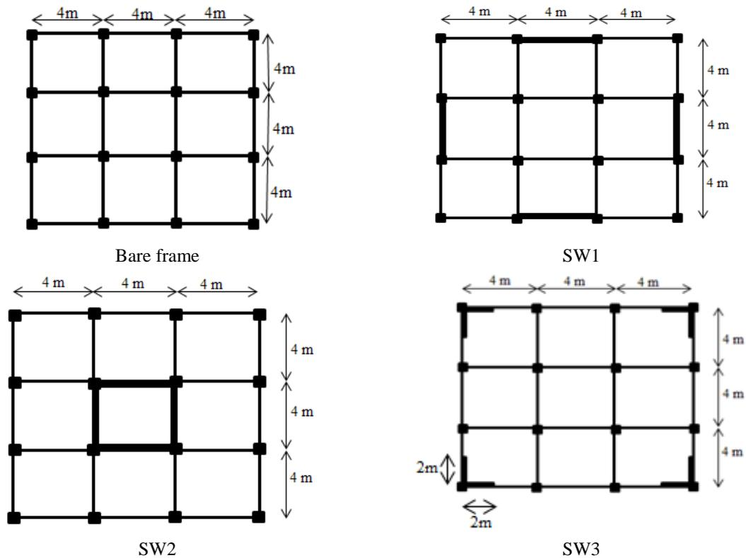
Fig. 9 Plan of bare frame and frames with various locations of shear wall
