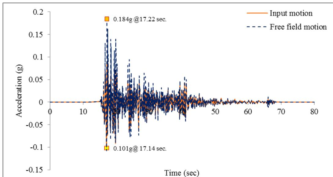
Fig. 5 Acceleration time history of free field motion at borehole 18
