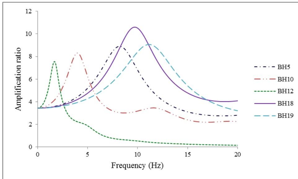
Fig. 8 Amplification ratio between surface and base motion
