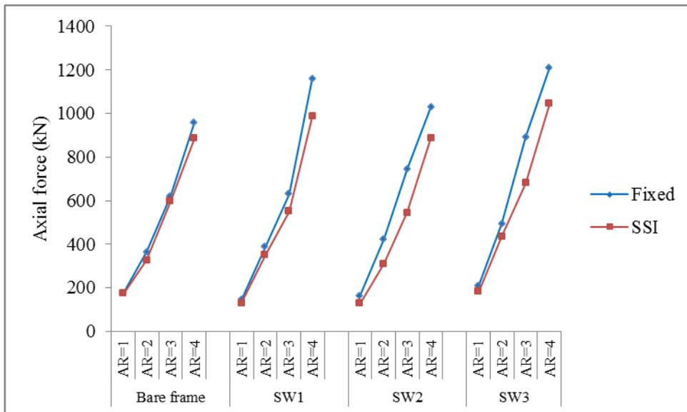
Fig. 14 Axial force in exterior column of ground floor
