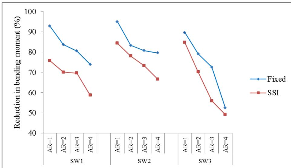
Fig. 16 Variation in bending moment in exterior column of ground floor
