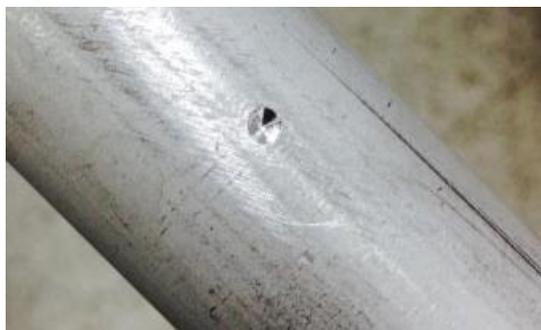
Fig. 2 A picture of the local sharp-notched circular tube
