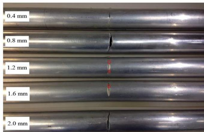
Fig. 19 A picture of the failure for sharp-notched 6061-T6 aluminum alloy circular tubes with  $a = 0.4, 0.8, 1.2, 1.6$  and  $2.0$  mm under cyclic bending
