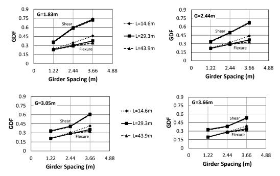
Fig. 5 Finite-element GDF versus girder spacing for the single lane trailer
