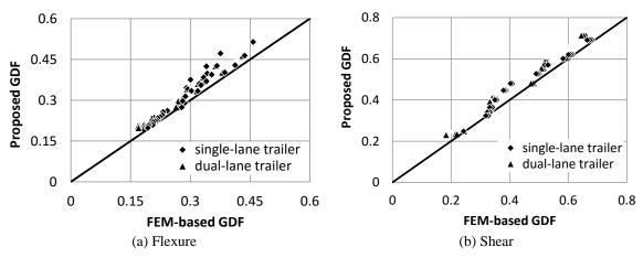
Fig. 7 Accuracy of the proposed GDF equations for flexure and shear
