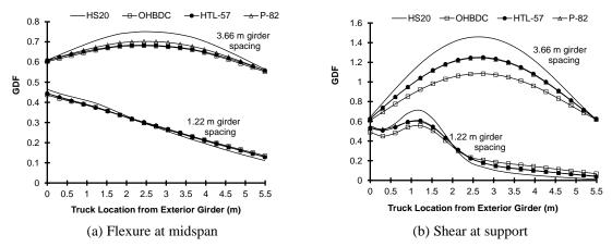
Fig. 3 Truck configuration effect on GDF for the 29.3 m long bridge and 1.83 m gage width
