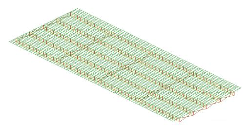
Fig. 4 Finite element model of a 29.3 m long bridge with 5 girders at 2.44 m spacing
