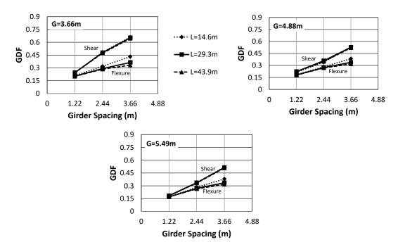
Fig. 6 Finite-element GDF versus girder spacing for the dual lane trailer
