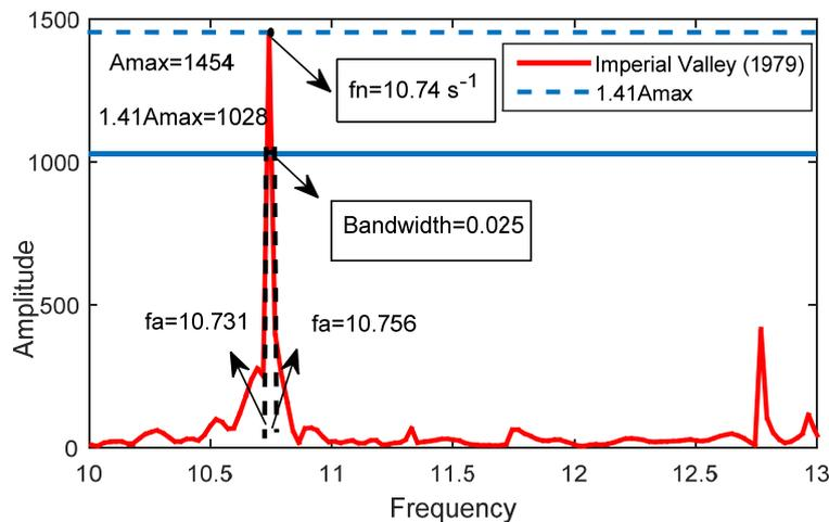
Fig. 16 Vertical damping estimation using Imperial Valley (1979)
