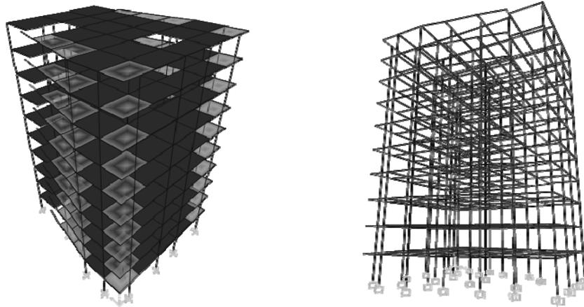
Fig. 4 3-D Finite element model of the structure
