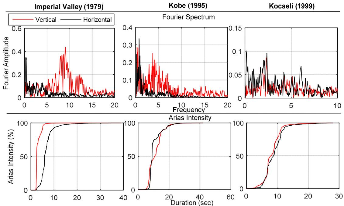
Fig. 2 Analysis of the vertical components of the earthquakes
