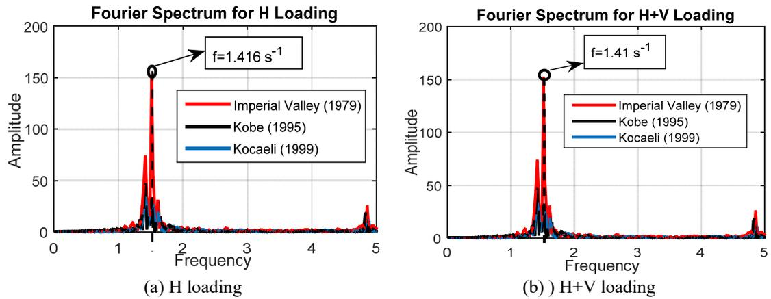
Fig. 13 FFT of lateral response acceleration data
