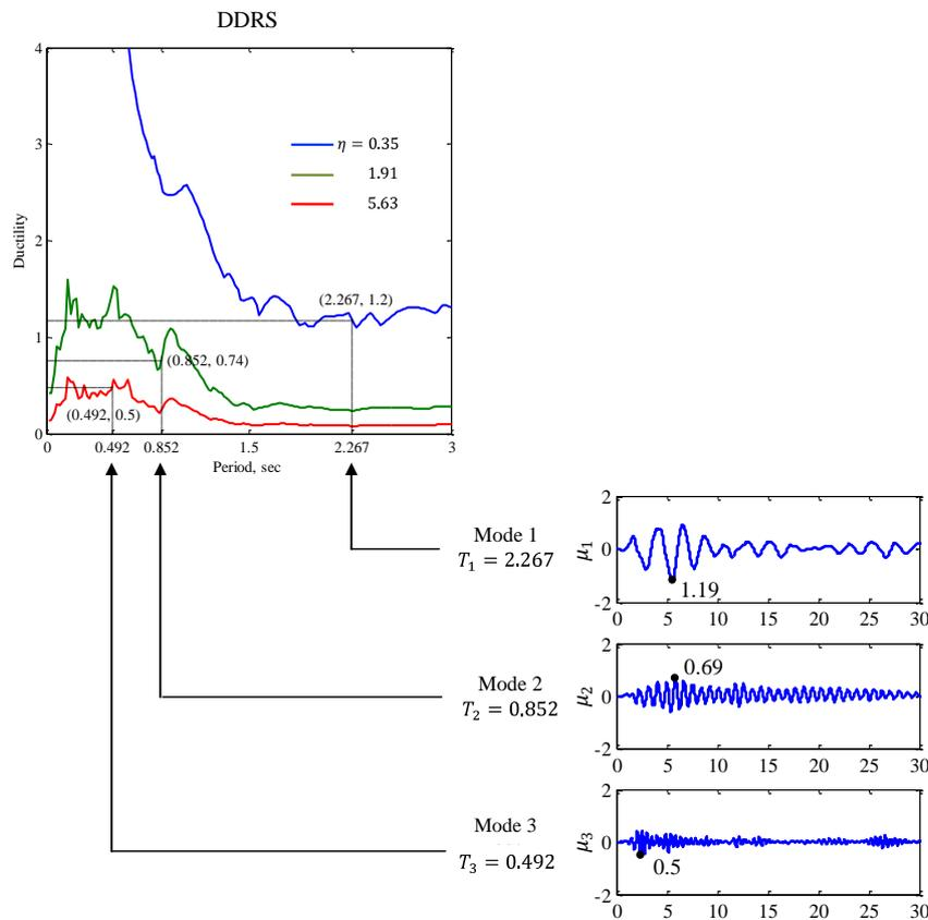
Fig. 7 Peak response of ductility demand from the DDRS spectra and the AMDA procedure for  $1.5 \times EI$  Centro ground motion: first three modal responses
