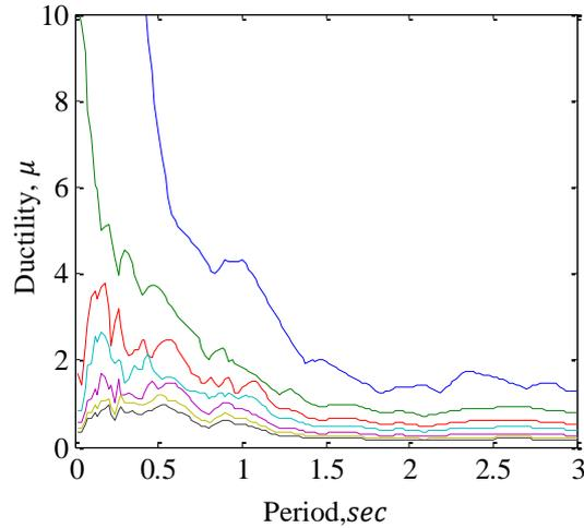
Fig. 6 DDRS for inelastic system computed for El Centro 1940 (N/S) component ( $\eta=0.25, 0.5, 0.75, 1, 1.5, 2, 2.5$  from top line to bottom line)
