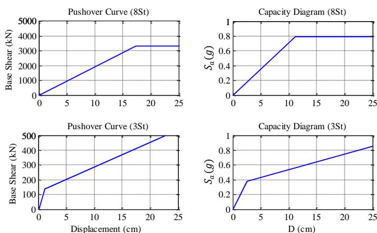
Fig. 9 Pushover curve and capacity diagram of the 1<sup>st</sup> mode for the 8St and the 3St structures
