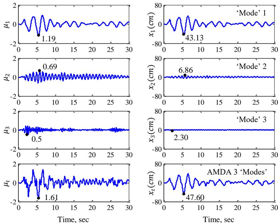
Fig. 4 Response histories of ductility demand and roof displacement from the proposed procedure for 1.5×El Centro ground motion: first three modal responses and total (all modes) response
