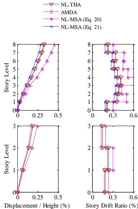
Fig. 12 Displacements and inter-story drifts ratio along the elevation for the 8St and the 3St buildings, obtained by the NL-THA, AMDA, NL-MSA (Eq.20) and NL-MSA (Eq.21) for LMSR ensemble
