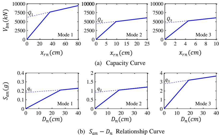
Fig. 3 Modal Pushover curves and capacity diagrams for the first three modes
