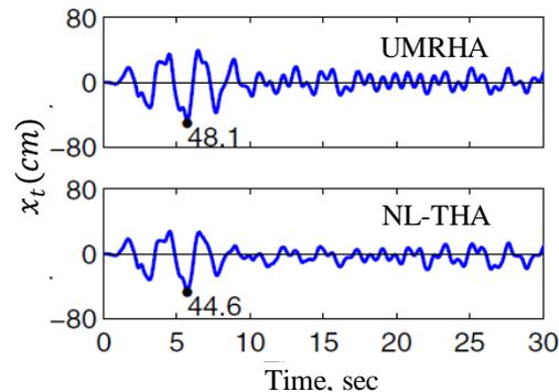
Fig. 5 Total response histories of roof displacement for  $1.5 \times \text{El Centro}$  ground motion from the UMRHA and NL-THA (Chopra and Goel 2001)
