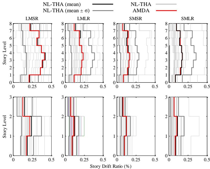
Fig. 11 Inter-story drift ratio obtained by the AMDA and NL-THA for the four ensembles
