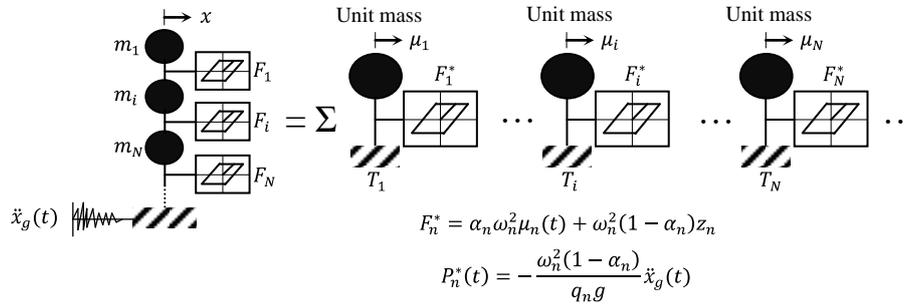
Fig. 2 Approximate multimodal dynamic procedure for MDOF structures
