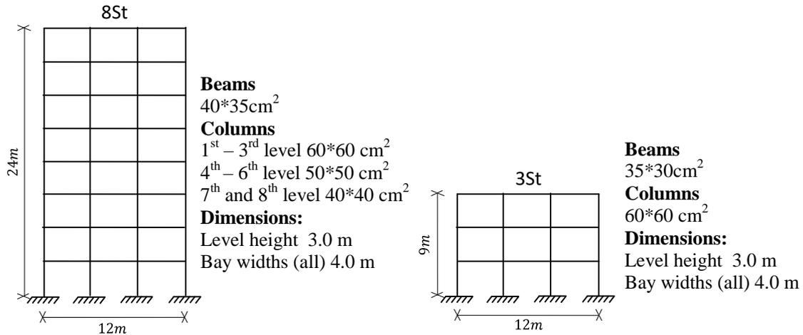
Fig. 8 Elevation view of the 8St and 3St structures
