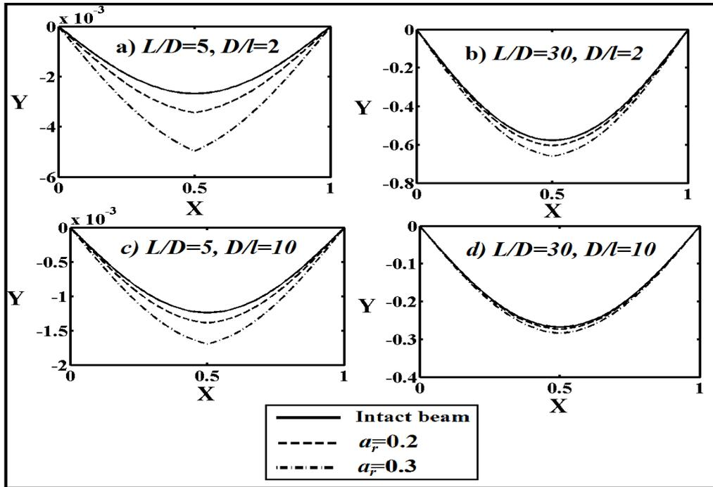
Fig. 11 The effect of the  $a_r$  on the deflected shape of the simple supported micro beam for (a)  $L/D=5$ ,  $D/l=2$ , (b)  $L/D=30$ ,  $D/l=2$ , (c)  $L/D=5$ ,  $D/l=10$ , (d)  $L/D=30$ ,  $D/l=10$
