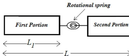
Fig. 2 Rotational spring model
