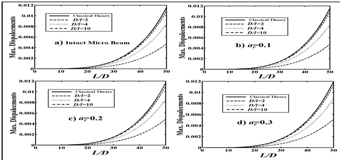
Fig. 7 Maximum vertical displacements of edge cracked simple supported micro beam with different the  $a_r$  and the  $L/D$  for  $q=10\mu\text{N}/\mu\text{m}$  and  $\eta=0.5$
