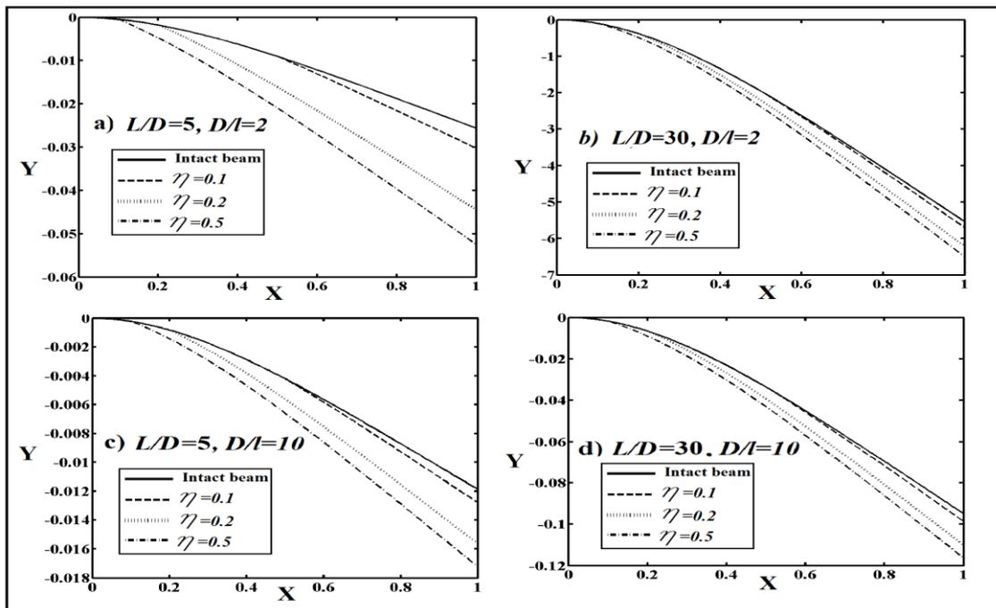
Fig. 12 The effect of the  $\eta$  on the deflected shape of the cantilever micro beam for (a)  $L/D=5$ ,  $D/l=2$ , (b)  $L/D=30$ ,  $D/l=2$ , (c)  $L/D=5$ ,  $D/l=10$ , (d)  $L/D=30$ ,  $D/l=10$
