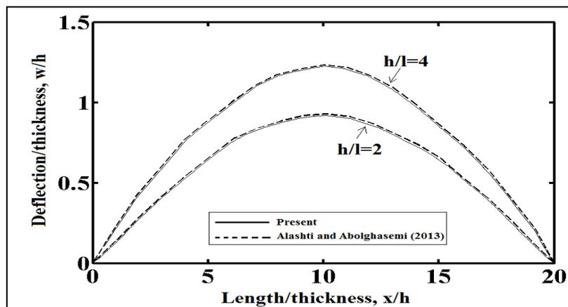
Fig. 5 Deflections of the simple supported beam based on the MCST
