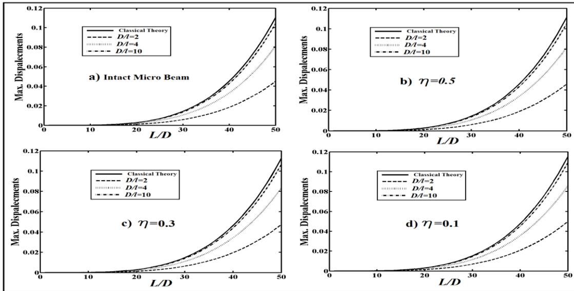
Fig. 8 Maximum vertical displacements of edge cracked cantilever micro beam with different the  $\eta$  and the  $L/D$  for  $q=10\mu\text{N}/\mu\text{m}$  and  $a_r=0.3$
