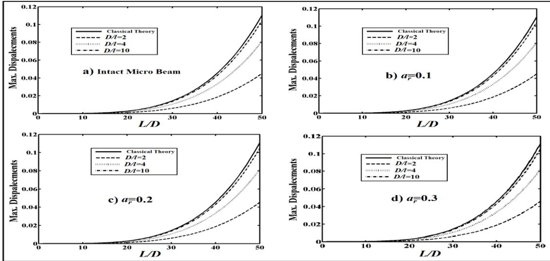
Fig. 6 Maximum vertical displacements of edge cracked cantilever micro beam with different the  $a_r$  and the  $L/D$  for  $q=10\mu\text{N}/\mu\text{m}$  and  $\eta=0.5$
