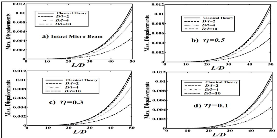
Fig. 9 Maximum vertical displacements of edge cracked simple supported micro beam with different the  $\eta$  and the  $L/D$  for  $q=10\mu\text{N}/\mu\text{m}$  and  $a_r=0.3$
