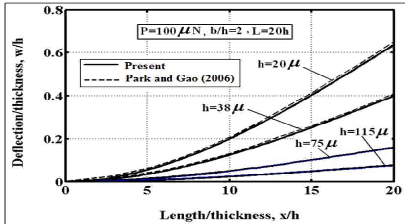
Fig. 4 Deflections of the cantilever beam based on the MCST
