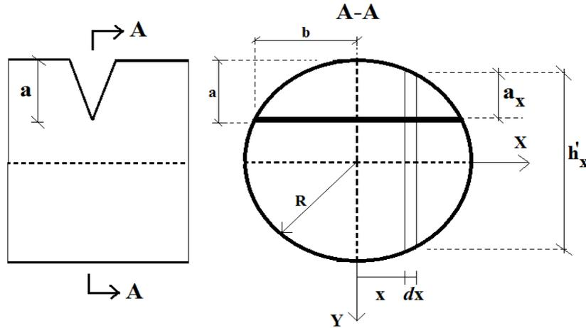
Fig. 3 The geometry of the cracked circular cross section
