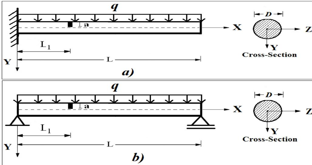
Fig. 1 Edge cracked circular micro beams with an open edge crack subjected to uniformly distributed transverse load ( $q$ ) and cross-section. (a) Cantilever micro beam, (b) Simple supported micro beam
