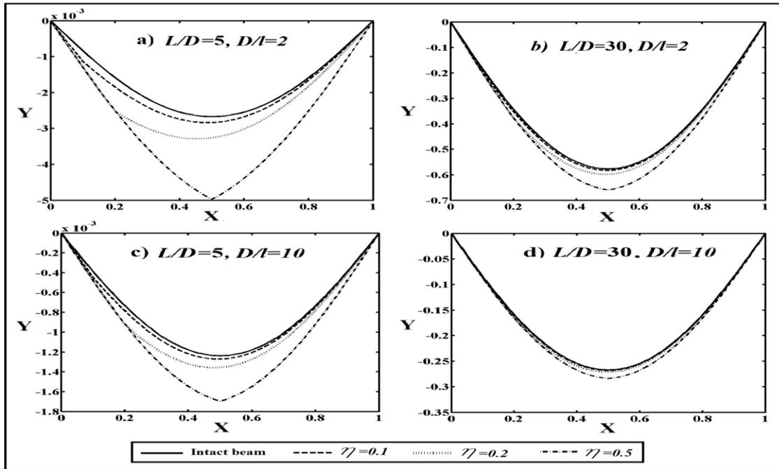
Fig. 13 The effect of the  $\eta$  on the deflected shape of the simple supported micro beam for (a)  $L/D=5$ ,  $D/l=2$ , (b)  $L/D=30$ ,  $D/l=2$ , (c)  $L/D=5$ ,  $D/l=10$ , (d)  $L/D=30$ ,  $D/l=10$
