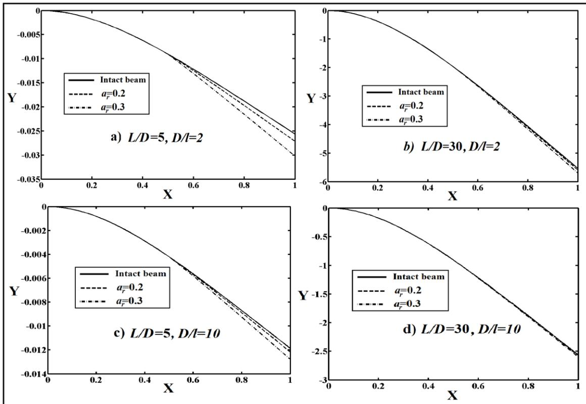
Fig. 10 The effect of the  $a_r$  on the deflected shape of the cantilever micro beam for (a)  $L/D=5$ ,  $D/l=2$ , (b)  $L/D=30$ ,  $D/l=2$ , (c)  $L/D=5$ ,  $D/l=10$ , (d)  $L/D=30$ ,  $D/l=10$
