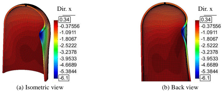
Fig. 13 Lateral displacements (cm) at 0.25 s. (magnification factor: 120)
