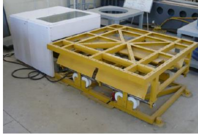
Fig. 1 General view of the shake table used for the tests
