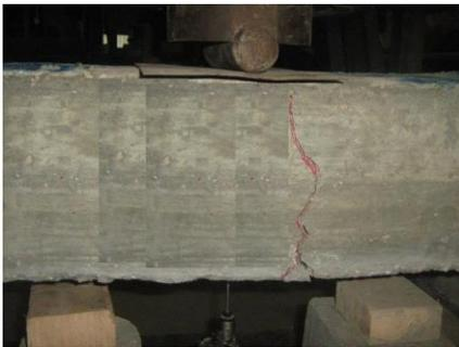
(a) Pattern of cracks shape of failure for beam (PC)
