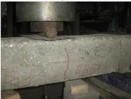
(c) Pattern of cracks, shape of failure for beam (FRP)
