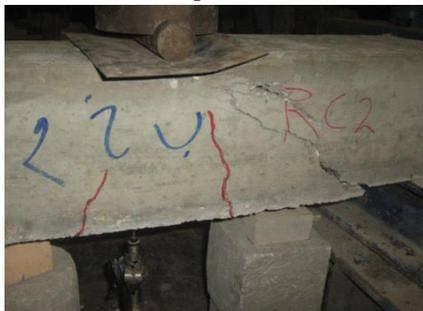
(e) Pattern of cracks, shape of failure of beam (RC)
