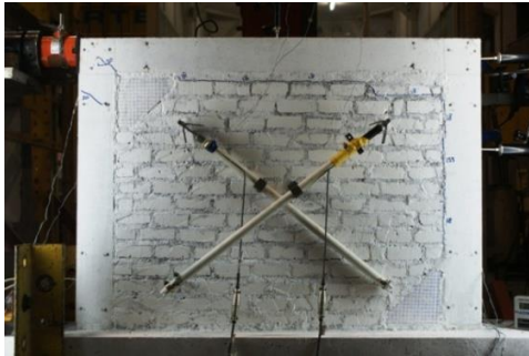
(c) First crack in the frame at 18.8 kN drift 0.24%
