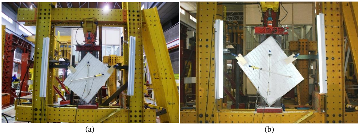
Fig. 7 Setup of (a) W1 and (b) W2 specimens for diagonal shear strength test
