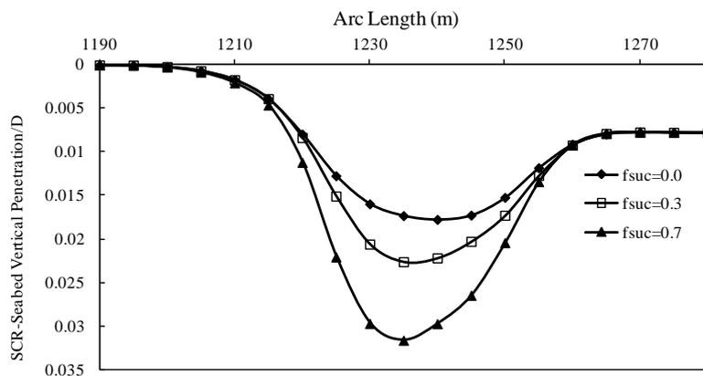
Fig. 19 Final trench profile for various values of the suction ratio
