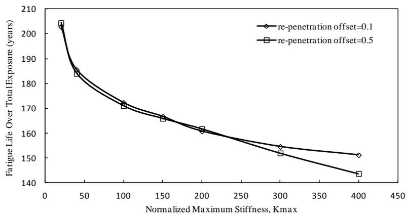
Fig. 17 Influence of normalised re-penetration offset on the predicted fatigue life
