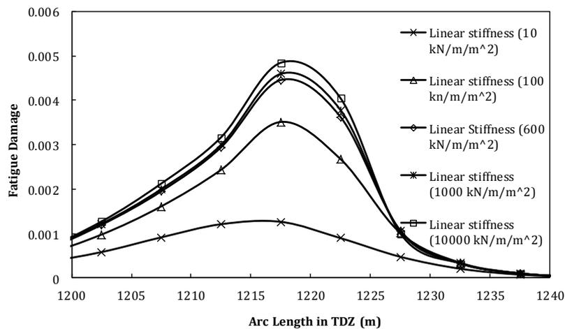
Fig. 10 Effect of linear soil stiffness on SCR cumulative fatigue damage in the TDZ
