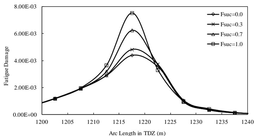
Fig. 15 Cumulative fatigue damage for different suction ratios in the TDZ ( $K_{max}=200$ )
