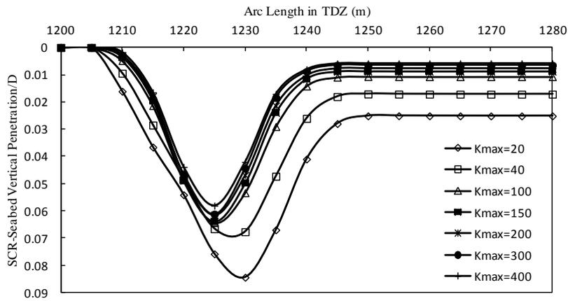
Fig. 14 Normalised maximum stiffness effect on trench deepening in the TDZ
