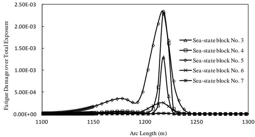
Fig. 9 Fatigue damage over total exposure for worst sea-state block (linear scale)
