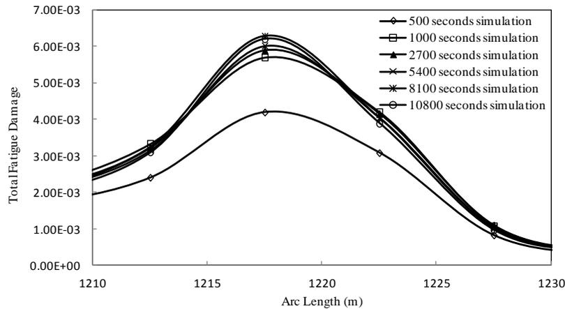
Fig. 18 Cumulative fatigue damage under different simulation time lengths (linear scale)
