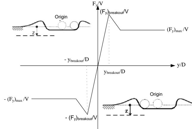
Fig. 3 Lateral pipe-soil interaction using a tri-linear model
