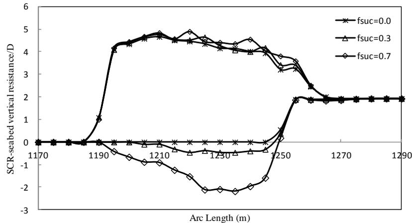
Fig. 20 Seabed resistance envelope for a range of suction values
