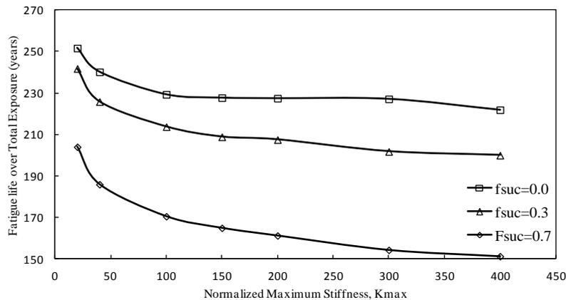
Fig. 16 Influence of maximum normalised stiffness and soil suction ratio on the predicted fatigue life
