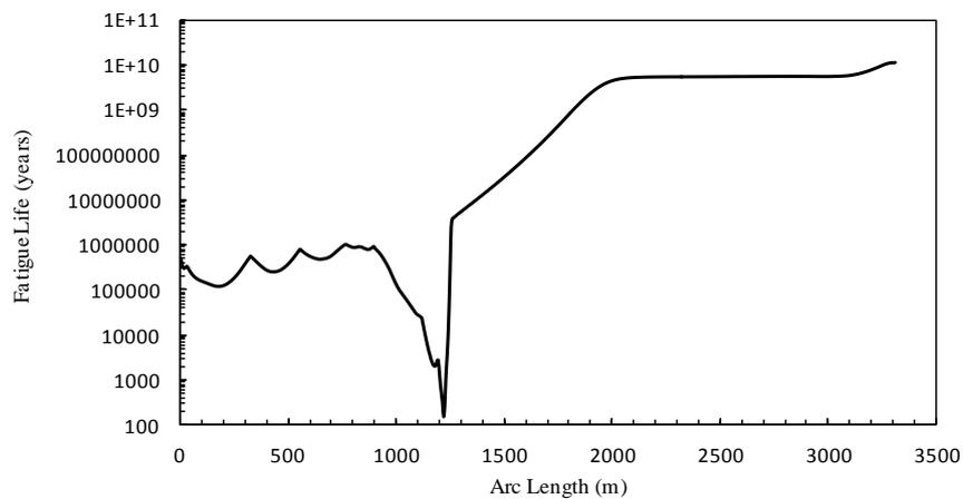
Fig. 8 Fatigue life along the SCR arc length measured from vessel with improved model
