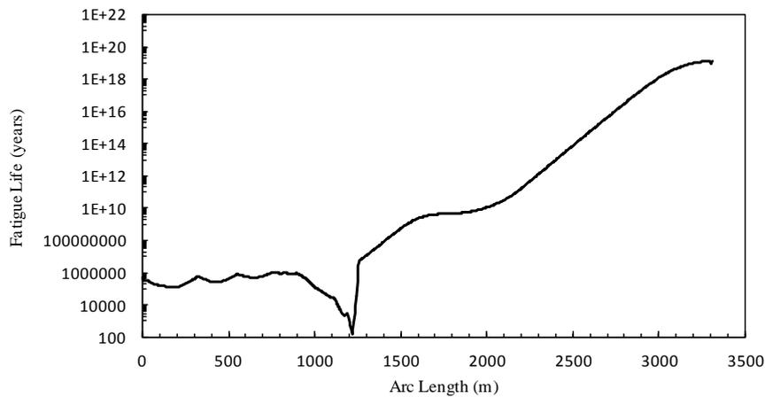
Fig. 7 Fatigue life along the SCR arc length measured from vessel with Coulomb model
