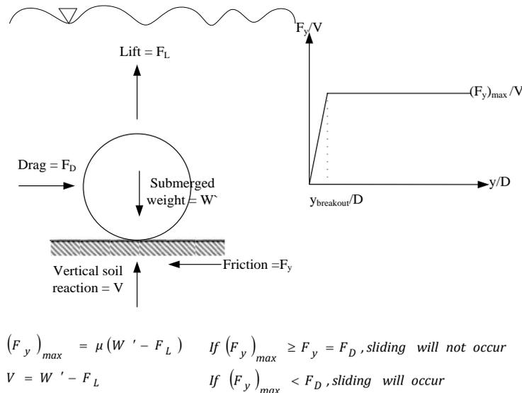
Fig. 2 Coulomb friction ‘bi-linear’ model
