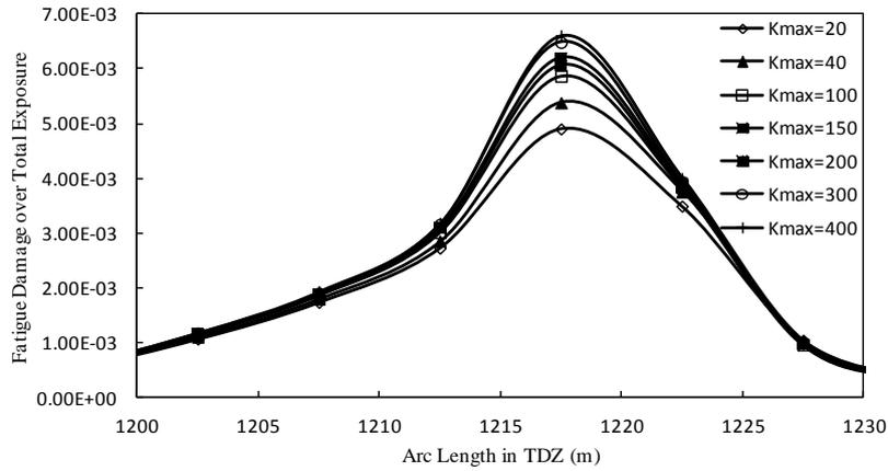
Fig. 12 Normalised maximum stiffness effect on fatigue damage in the TDZ
