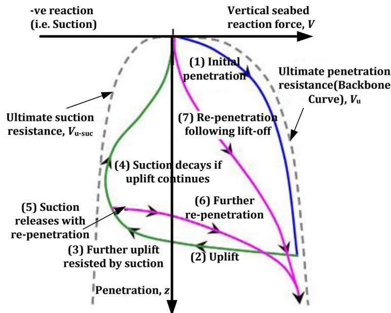
Fig. 1 Soil model characteristics for different modes (Randolph and Quiggin 2009)
