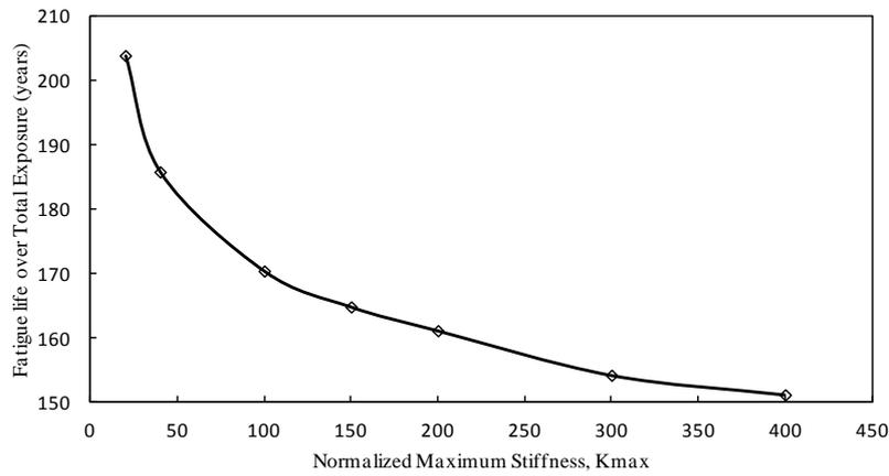
Fig. 13 Normalised maximum stiffness effect on fatigue life in the TDZ at arc length 1217.5 m
