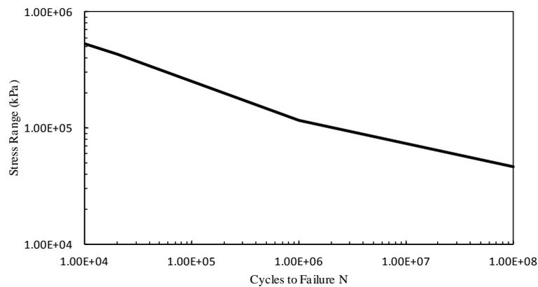
Fig. 4 An example of a DNV S-N curve (from DNV-RP-C203)
