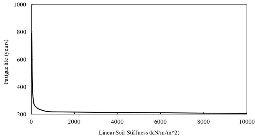
Fig. 11 Linear seabed model: soil stiffness effect on predicted fatigue life
