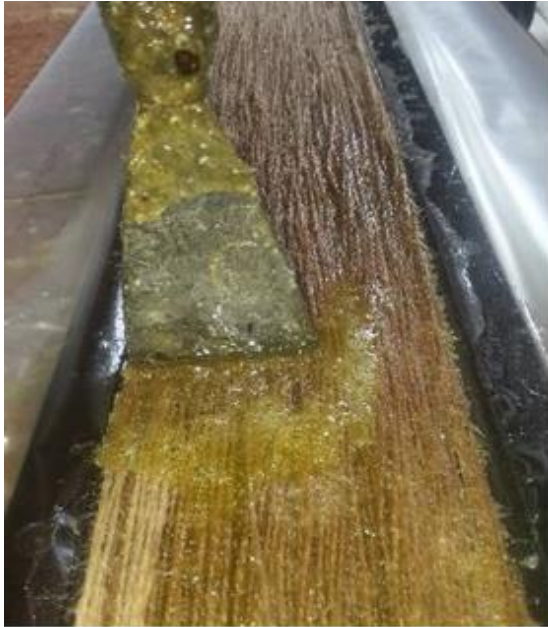
Fig. 3(a) Spreading adhesive
