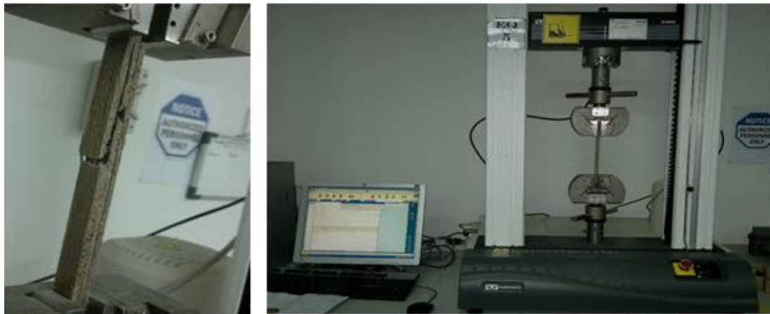
Fig. 4 Universal testing machin INSTRON for tensile test
