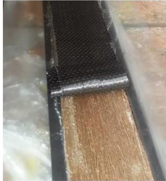
Fig. 3(b) Applying carbon fiber on jute ropes
