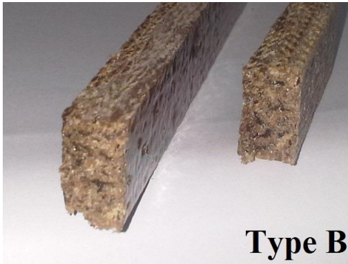
Fig. 7 Rapture of fabricated plates type A and B after tensile test
