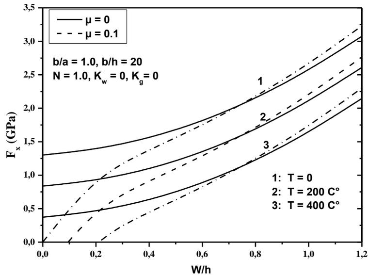
Fig. 12 Effects of the temperature field on the post-buckling of FG plates under uniaxial compression (immovable on  $y=0, b$ )
