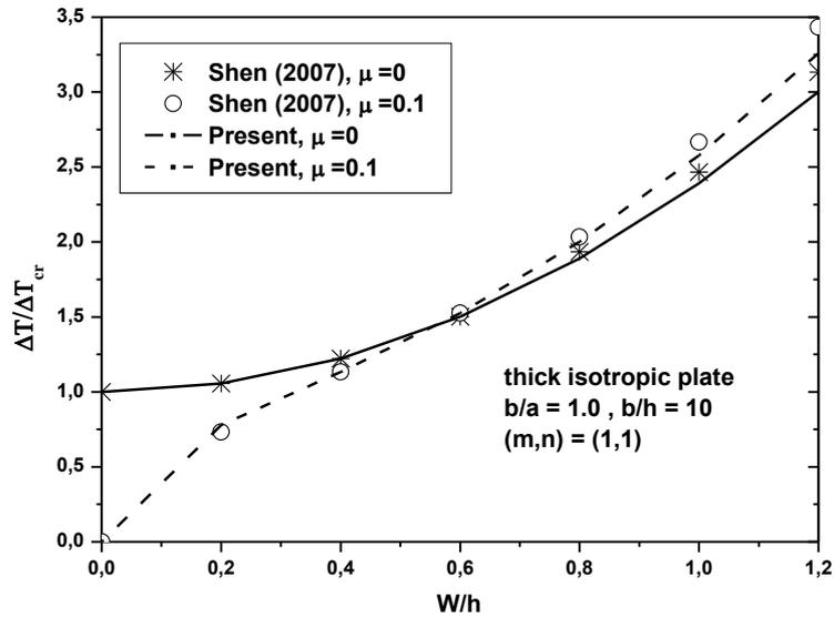
Fig. 2 Comparisons of thermal post-buckling load-deflection curves for isotropic plates
