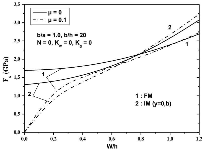
Fig. 4 Effects of in-plane restraint on the post-buckling of FG plate under uniaxial compression
