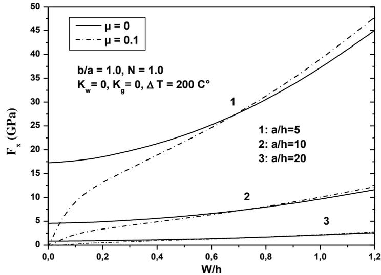
Fig. 11 Effects of the thickness ratios on the post-buckling of FG plates under uniaxial compression (immovable on  $y=0, b$ )
