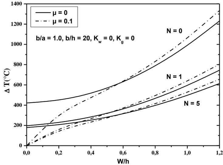
Fig. 5 Effects of the power law index on the post-buckling of FG plates under uniform temperature rise (all IM edges)
