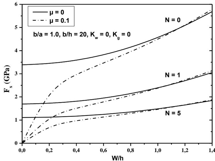
Fig. 3 Effects of the power law index on the post-buckling of FG plates under uniaxial compressive load (all movable edges)
