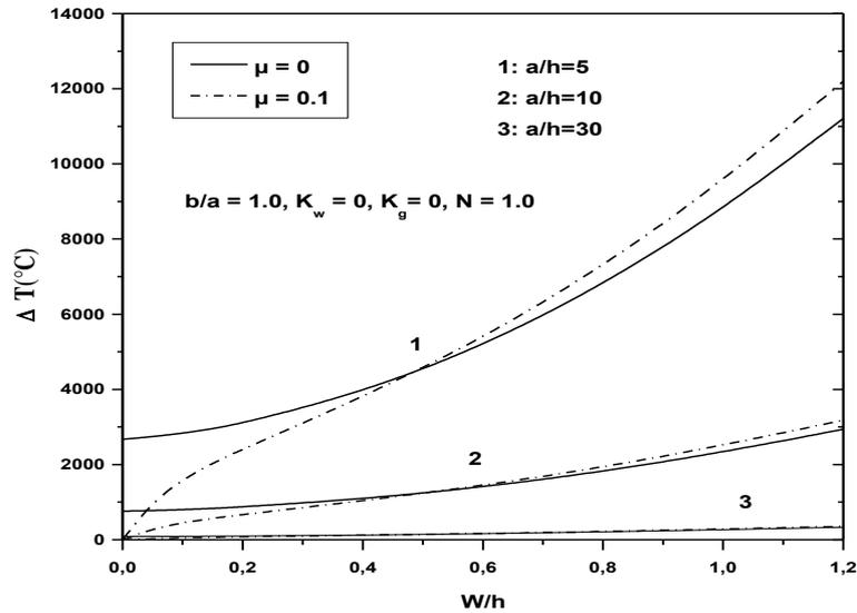
Fig. 9 Effects of the thickness ratios on the post-buckling of FG plates under uniform temperature rise (all IM edges)
