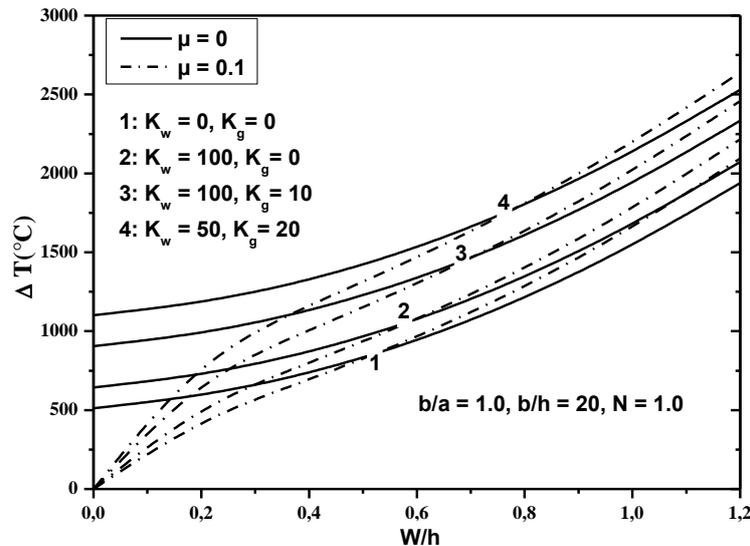
Fig. 8 Effects of the elastic foundations on the post-buckling of FG plates under temperature gradient (all IM edges)
