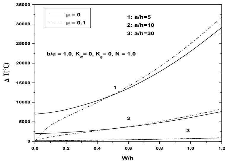
Fig. 10 Effects of the thickness ratios on the post-buckling of FG plates under temperature gradient (all IM edges)
