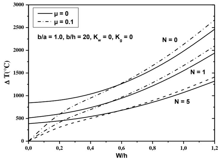
Fig. 6 Effects of the power law index on the post-buckling of FG plates under nonlinear temperature distribution (all IM edges)
