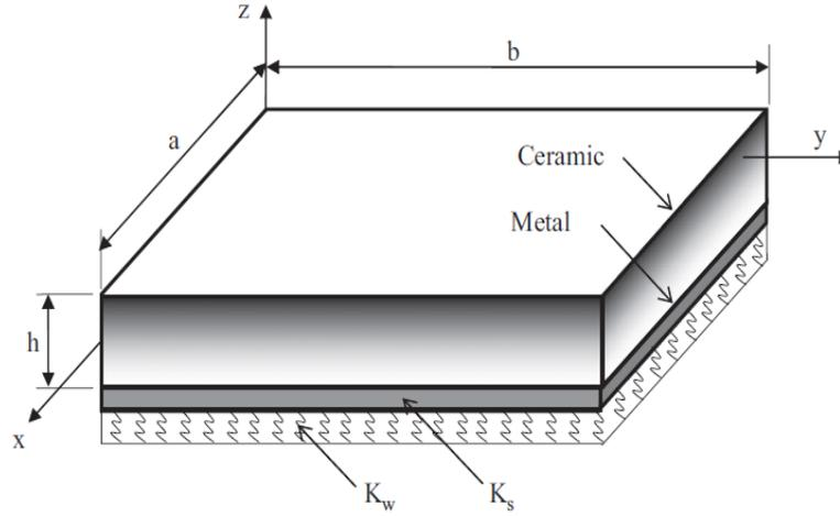
Fig. 1 Coordinate system and geometry for FG plates on Pasternak elastic foundation
