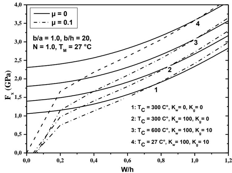
Fig. 13 Interactive effects of elastic foundation and nonlinear temperature distribution on the post-buckling of FG plates under uniaxial compression (immovable on  $y=0, b$ ).
