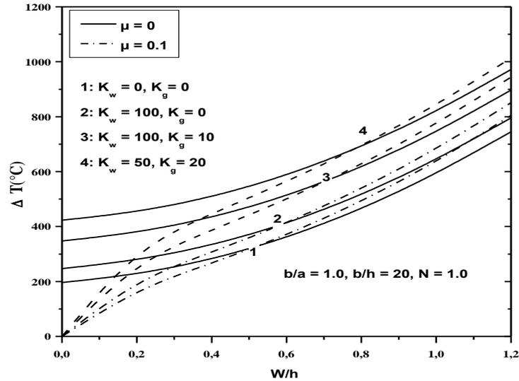
Fig. 7 Effects of the elastic foundations on the post-buckling of FG plates under uniform temperature rise (all IM edges)
