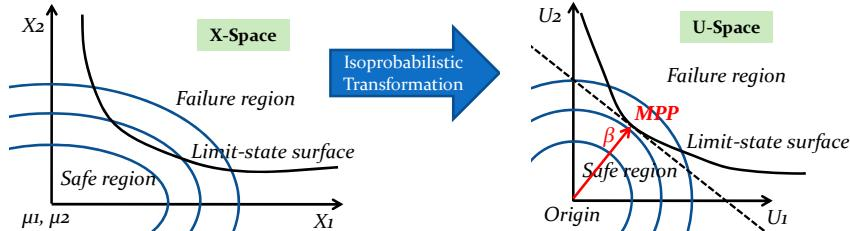
Fig. 1 Isoprobabilistic transformation and reliability measures
