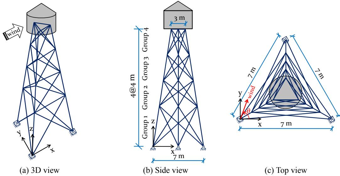
Fig. 10 Three-dimensional 39-bar truss
