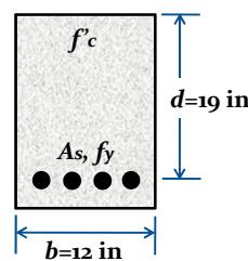
Fig. 7 Cross section of RC beam
