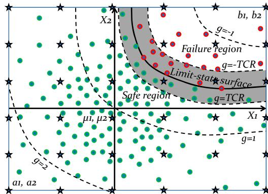
Fig. 3 Details of concepts of the proposed method for truncated random variables
