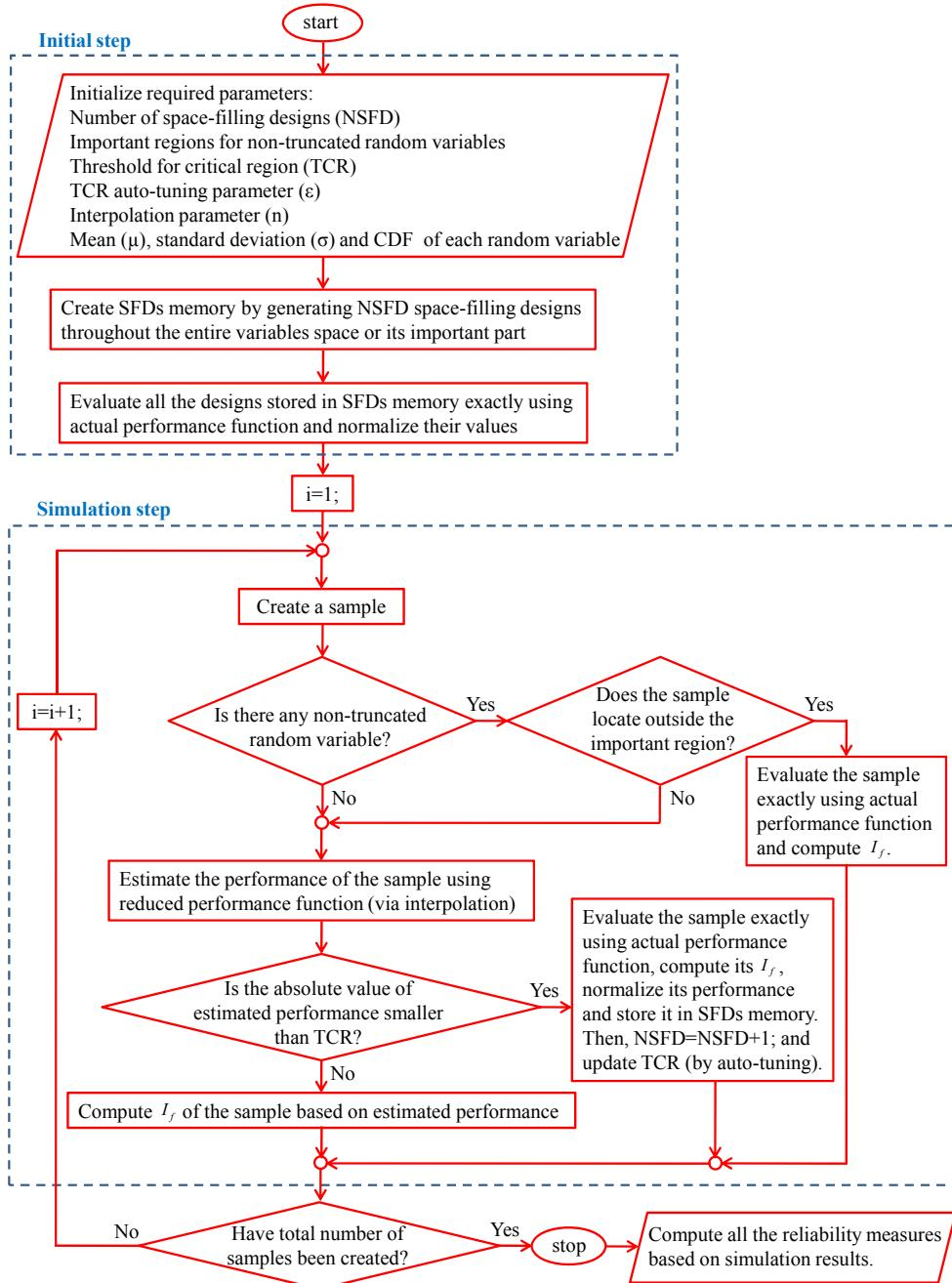
Fig. 5 The flowchart of the proposed reliability analysis method
