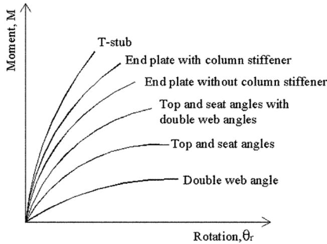
Fig. 2 Moment-rotation curves of semi-rigid connections
