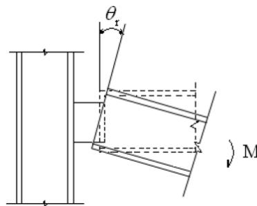
Fig. 1 Rotation of a semi-rigid connection
