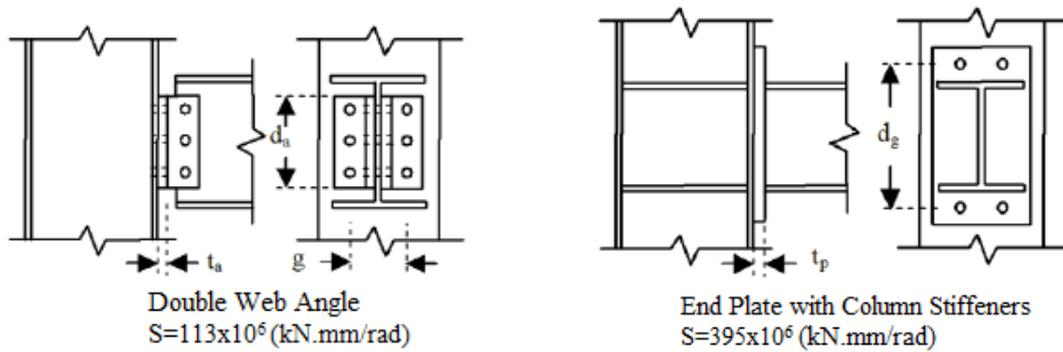
Fig. 3 The two types of connections and rotational stiffness values
