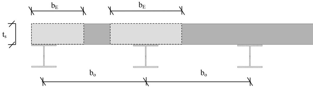
Fig. 4 Effective width of composite beam
