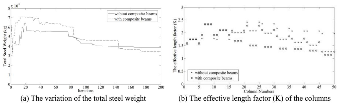
Fig. 12 Semi rigid steel frame with End Plate with Column Stiffness connection with and without composite beams
