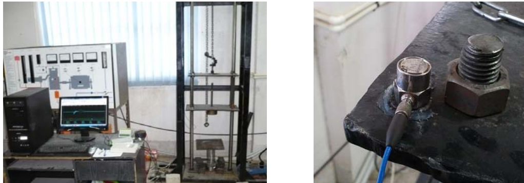
Fig. 3 Drop hammer apparatus and accelerometer sensors
