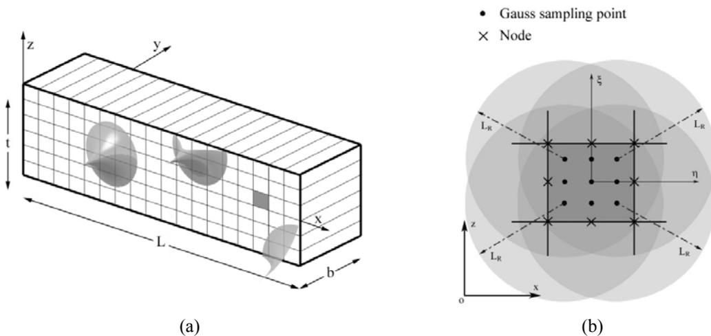
Fig. 5 Typical finite element mesh arrangement and typical element for a beam. (Pisano *et al.* 2009)
