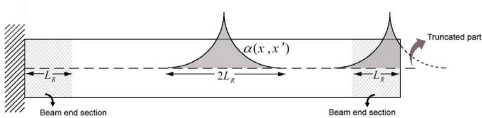
Fig. 1 Modification of kernel at beam end sections (Pisano *et al.* 2009)
