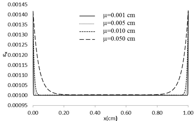
Fig. 3 Strain distribution for a bar in tension with various influence distance parameter
