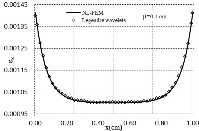
Fig. 2 Strain distribution for a bar in tension with NL-FEM (solid line) and Legendre wavelets method (points).  $\mu$  is the scale coefficient that incorporates the small-scale effect and is equal to  $l\tau$
