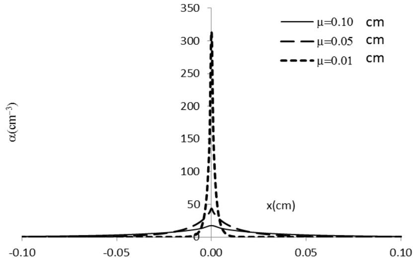
Fig. 4 Effects of  $\mu$  on attenuation function distribution
