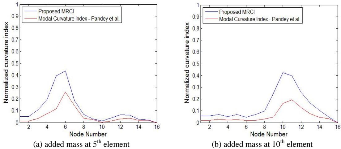
Fig. 7 The experimental results of mean of normalized MRCI and MCI proposed by Pandey *et al.* for the cases of the added mass at 5<sup>th</sup> and at 10<sup>th</sup> element individually.
