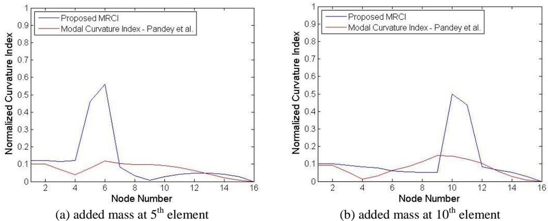
Fig. 6 The numerical results of mean of normalized MRCI and MCI proposed by Pandey *et al.* for the cases of the added mass at 5<sup>th</sup> and at 10<sup>th</sup> element individually
