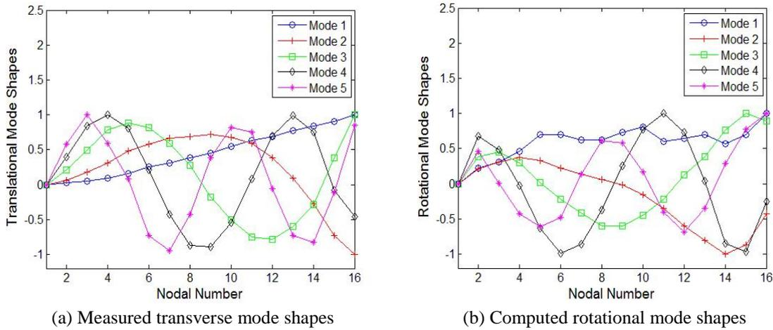
Fig. 4 Measured transverse mode shapes and computed rotational mode shapes for the undamaged case
