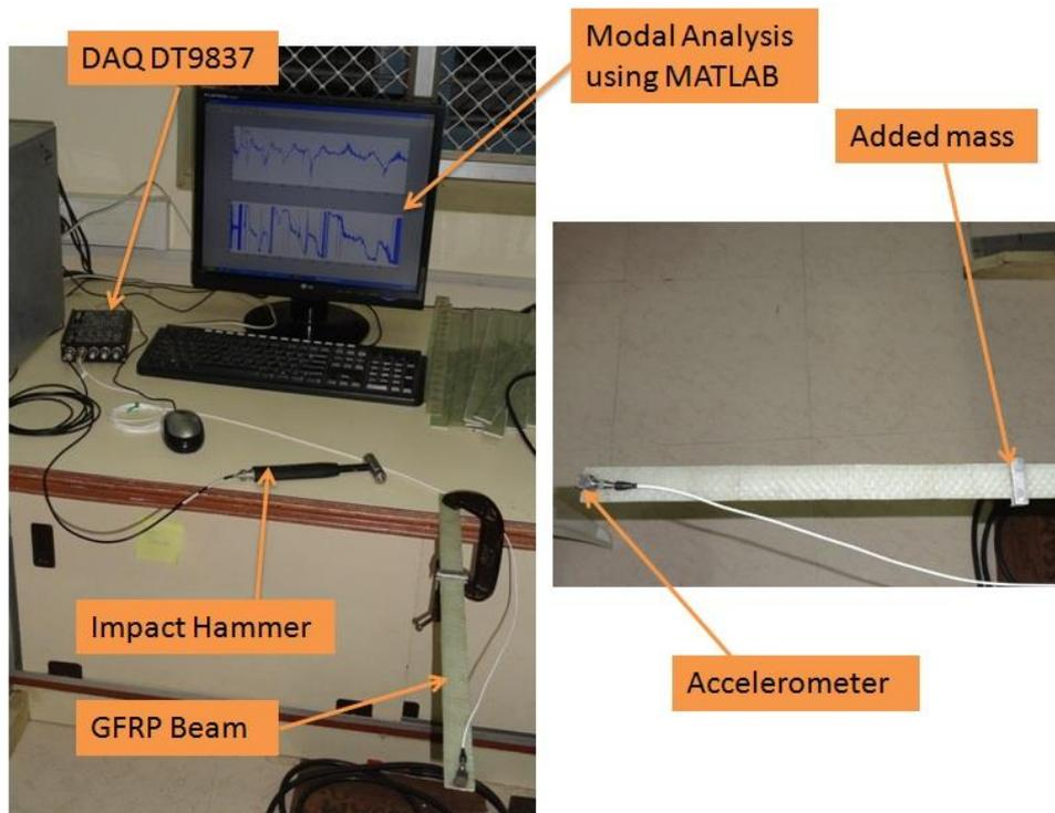
Fig. 3 (a) Experimental modal analysis test setup (b) Added mass is attached with GFRP beam
