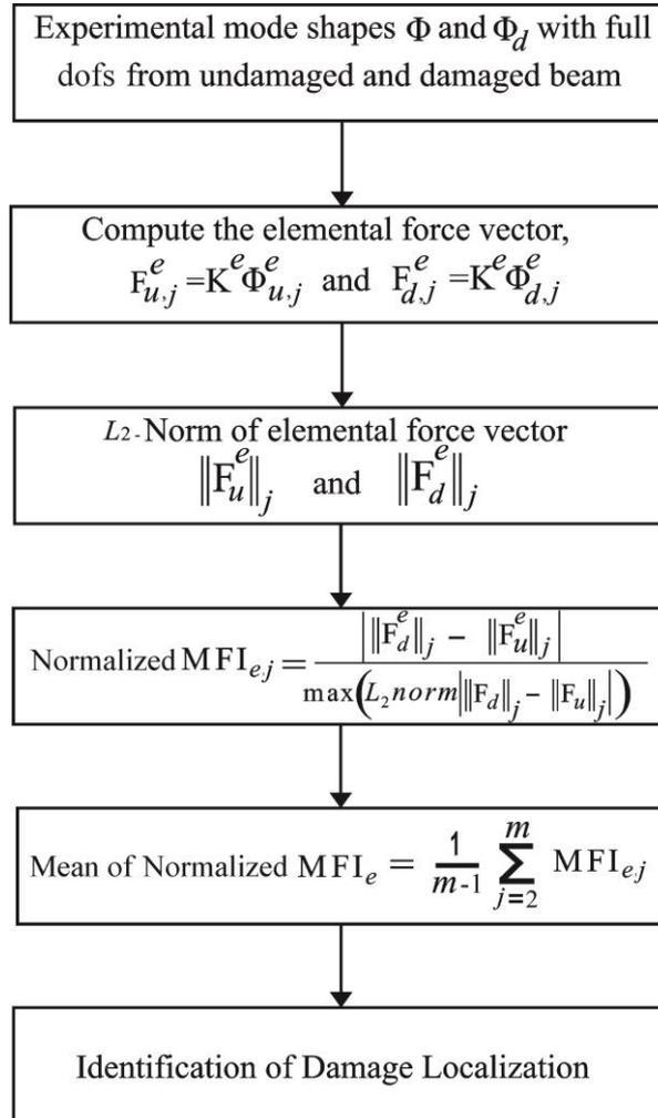
Fig. 1 Damage identification algorithm based on modal force index
