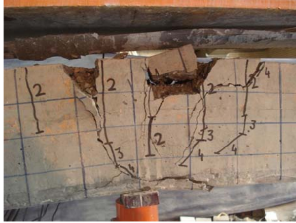
Fig. 10 Failure of beam E50NB (debonding accompanied with the concrete cover separation)
