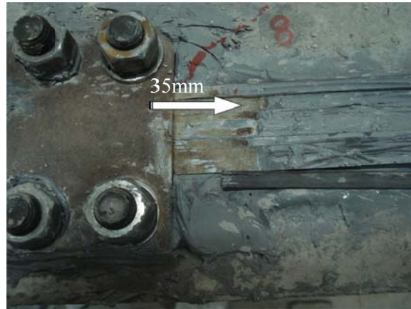
Fig. 8 End-anchorage failure of beam E50NA (laminates slipping)
