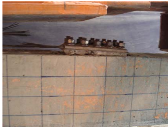
Fig. 9 End-anchorage failure of beam E30NB (end-anchorage pull-off and FRP rupture)
