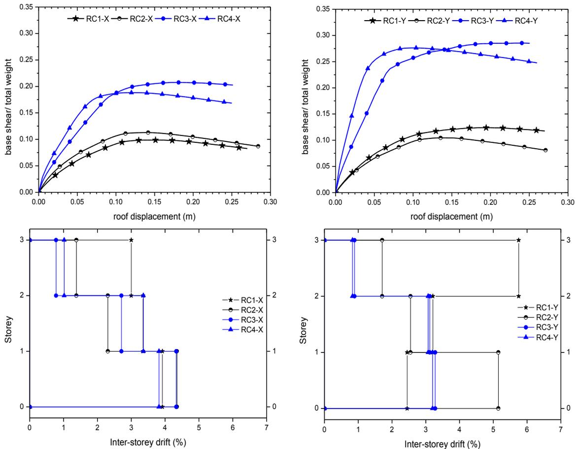
Fig. 14 Capacity curves and corresponding IS drift of NRCB1, NRCB2, NRCB3 and NRCB4 building structures with (a) longitudinal (X) and (b) transverse (Y) directions of loading
