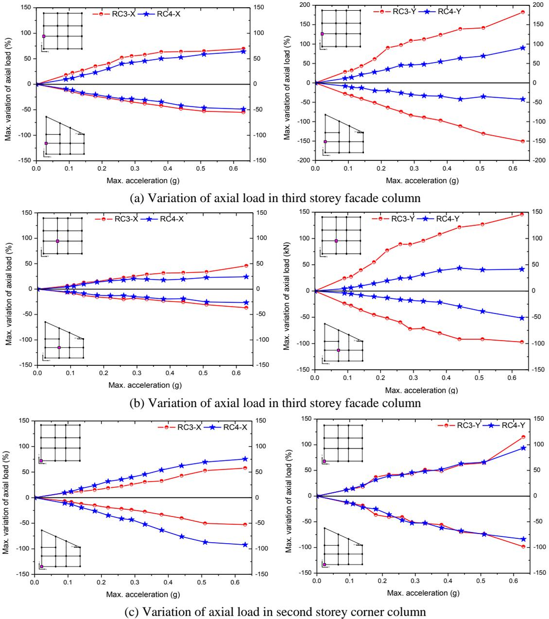
Fig. 21 Maximum variation of axial load for RC3 and RC4 building models in X and Y direction of loadings
