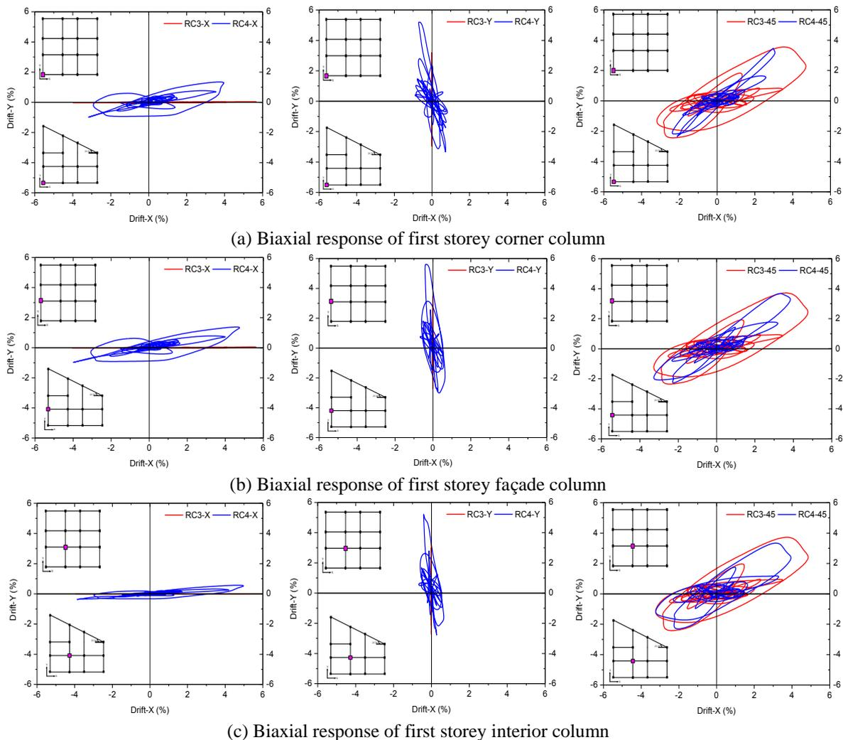
Fig. 20 Biaxial response of RC3 and RC4 building models in X, Y and 45° direction of loading condition
