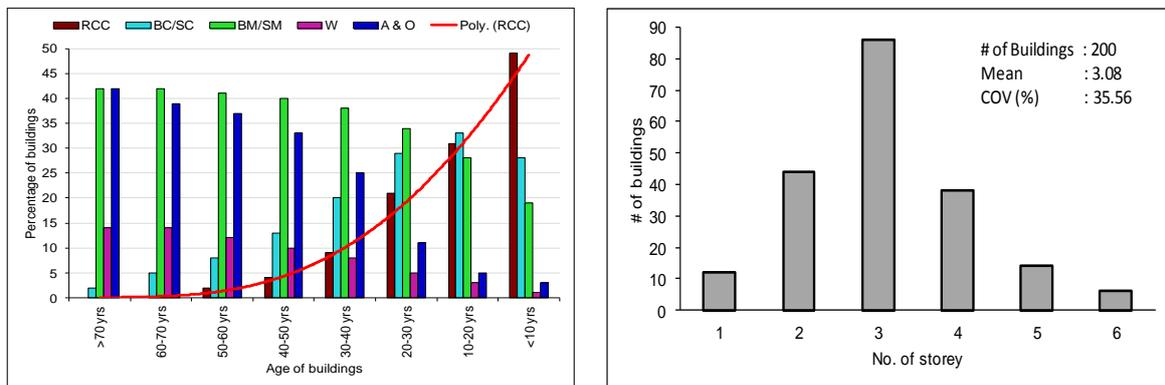
Fig. 5 Distribution of (a) age of RC buildings and (b) number of storey of RC buildings
