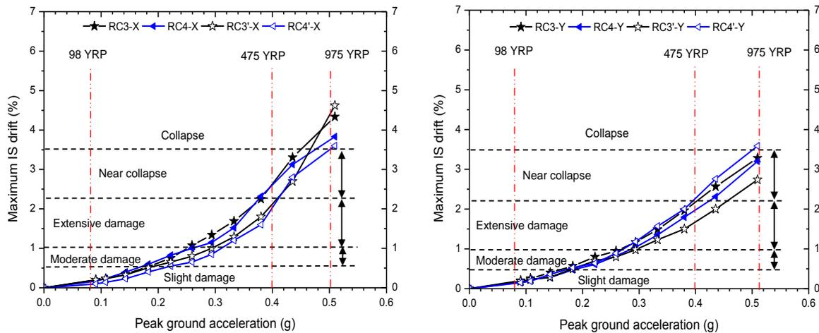
Fig. 19 Vulnerability curves of the maximum IS drift for RC3 and RC4 structures with and without P-delta effect for longitudinal (X) and transverse (Y) directions of loading
