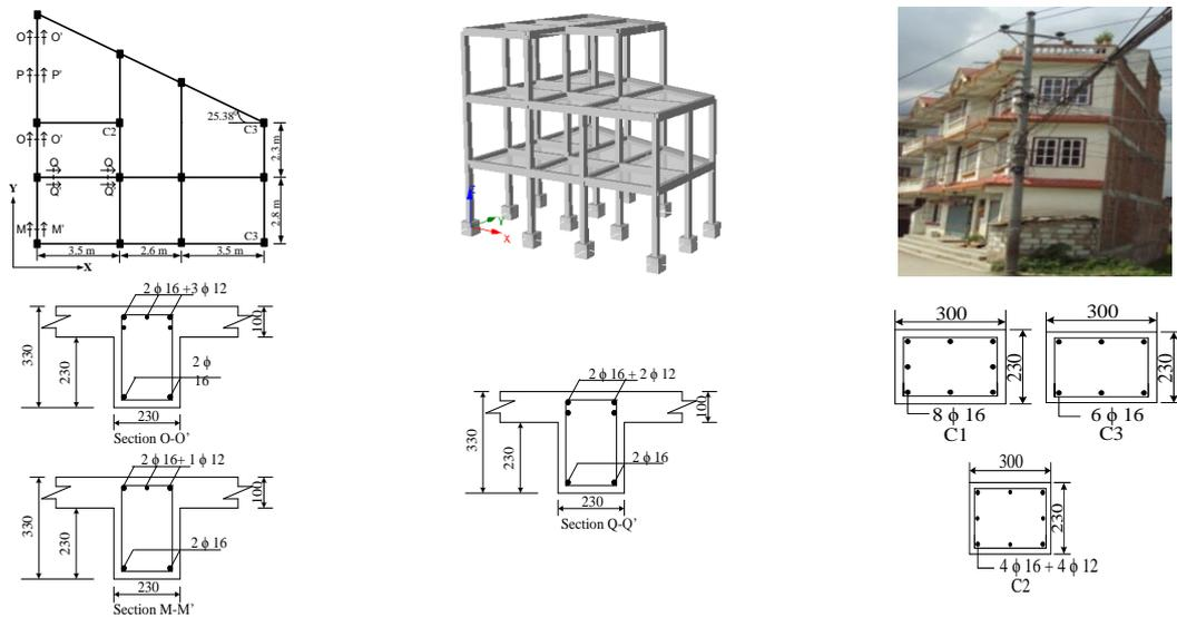
Fig. 13 Plan, tridimensional model, and cross-section detailing of building model RC4
