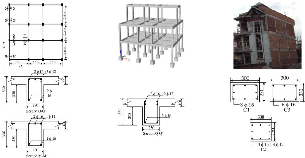
Fig. 12 Plan, tridimensional model, and cross-section detailing of building model RC3
