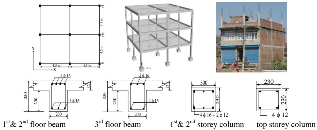
Fig. 10 Plan, tridimensional model, and cross-section detailing of building model RC1
