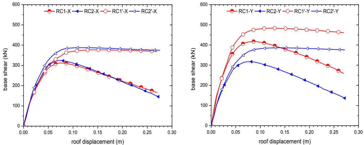
Fig. 16 The capacity curve and corresponding IS drift of the studied building structures with and without considering the  $P$ -Delta effect for longitudinal ( $X$ ) and transverse ( $Y$ ) directions of loading
