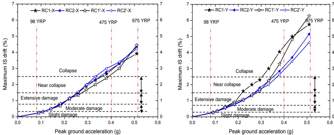
Fig. 18 Vulnerability curves of the maximum IS drift for RC1 and RC2 structures with and without  $P$ -delta effect for longitudinal (X) and transverse (Y) directions of loading
