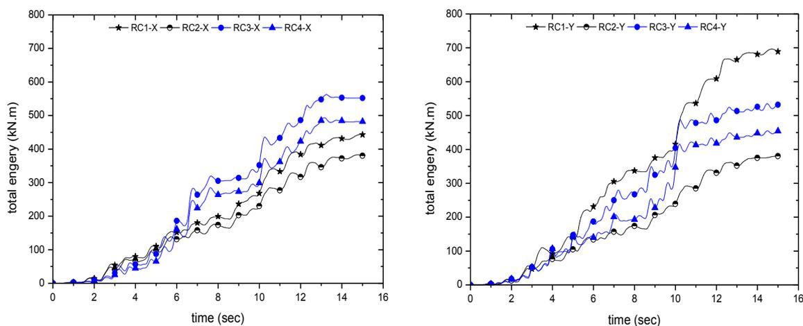
Fig. 15 Total energy dissipation profiles for existing building structures in Nepal
