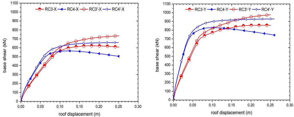
Fig. 17 The capacity curve and corresponding IS drift of the studied building structures with and without considering the *P*-Delta effect for longitudinal (*X*) and transverse (*Y*) directions of loading
