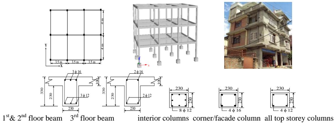
Fig. 11 Plan, tridimensional model, and cross-section detailing of building model RC2
