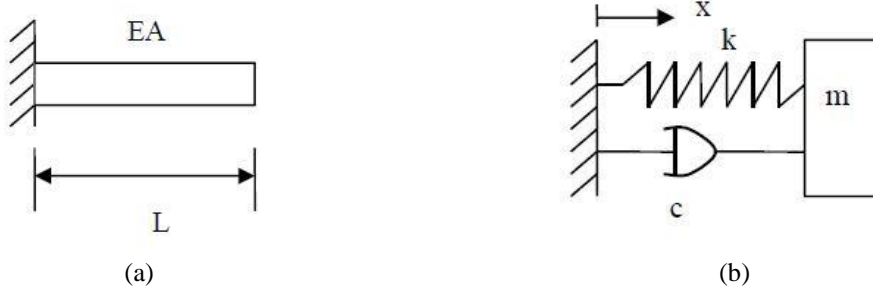
Fig. 1 (a) A cantilever bar, (b) The equivalent single DOF system
