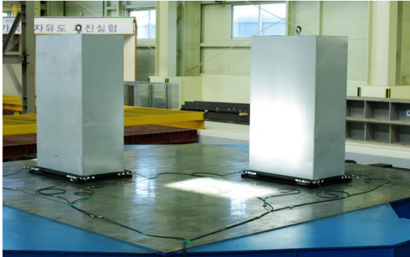
Fig. 11 CFPBS and sensors arrangement for the shaking table test
