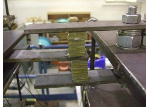
(c) Damper installed between models
