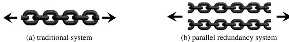
Fig. 1 Traditional and parallel redundancy systems
